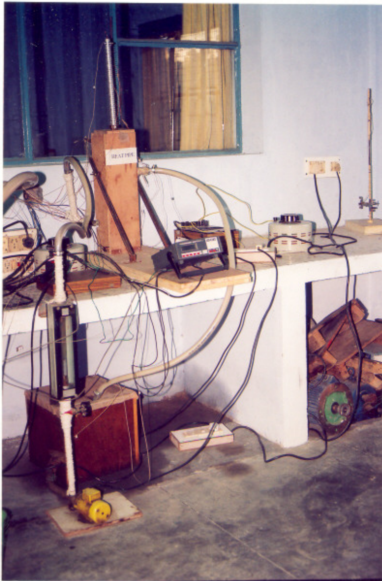
Plate 4.1: A test set up of single heat pipe under vertical condition
