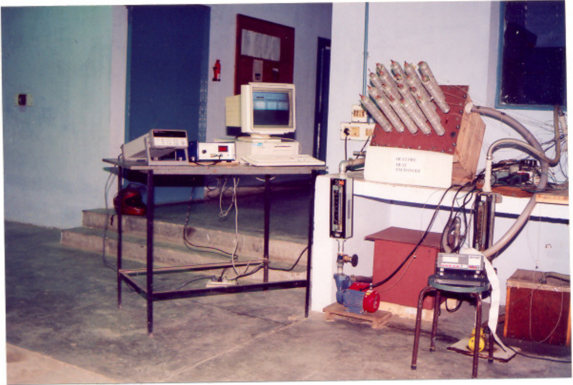
Plate 4.4: A test set up of HPHE under inclined condition
