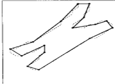
Figure 3.20 Teh-Chin algorithm (k curvature) [20].
