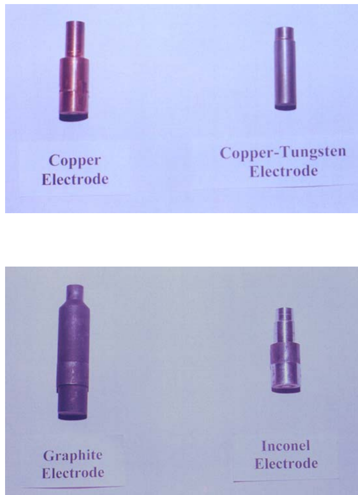
Fig. 4.1 Electrode materials used for experimentation
