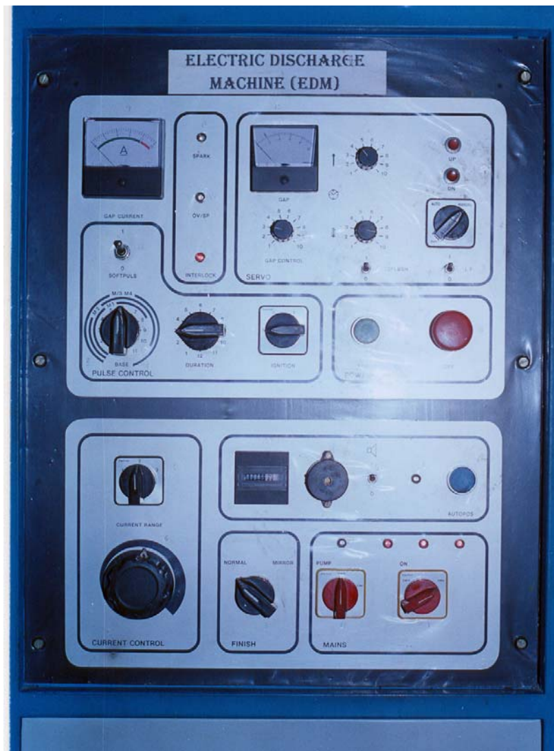
Fig. 3.2 Control Panel of the EDM machine
