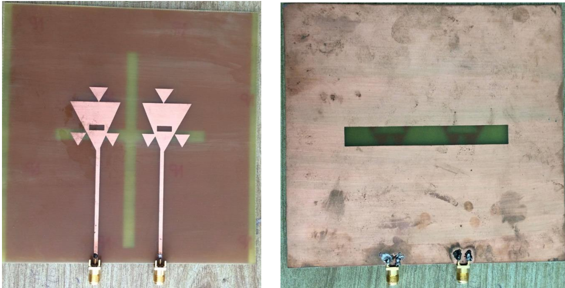
Figure 5.6 (a) Patch with microstrip feed line (b) DGS on ground plane
