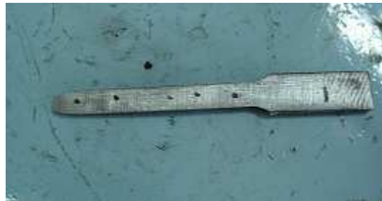
Fig 4.4 Analysis of tension specimen: fracture stage for Corten steel (sheet sample)
