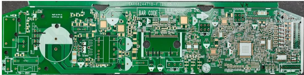
Figure 4.5 : Markings on PCB after silk screen print
