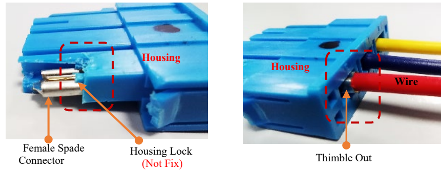
Figure 5.15: Housing Lock is not Fix
