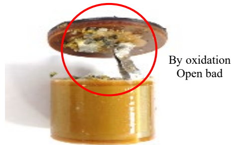
Figure 4.23: Disassembled photo of field defect capacitor
