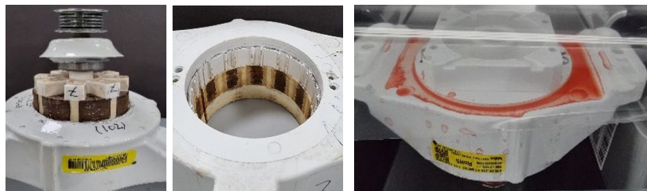
Figure 5.13: BLDC motor shaft, rusted rotor and water at bottom of motor
