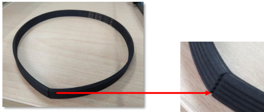
Figure 5.18: Motor V-Belt damaged
