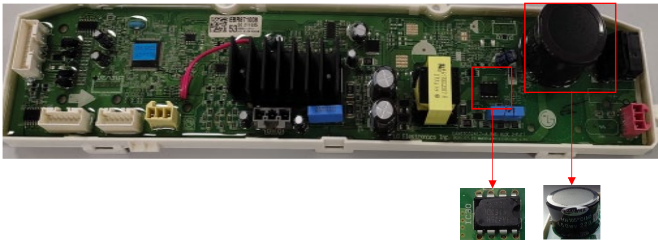
Figure 4.3: SMPS IC and DC link capacitor
