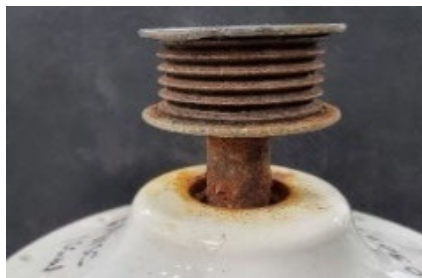
Figure 5.11: Rust on motor pulley
