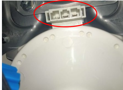
Figure 5.4: Motor Terminal Pin bend
