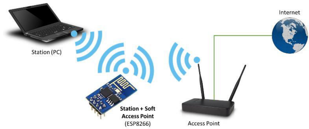
Fig.4.4 ESP8266 in station + soft access point mode
