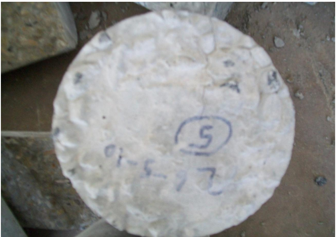
Fig 7.25: Failure pattern of plastic concrete
