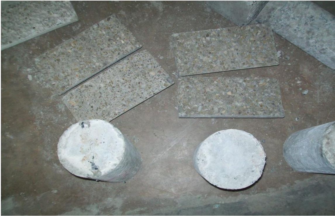
Fig 7.24: Showing failure pattern of control and plastic concrete.
