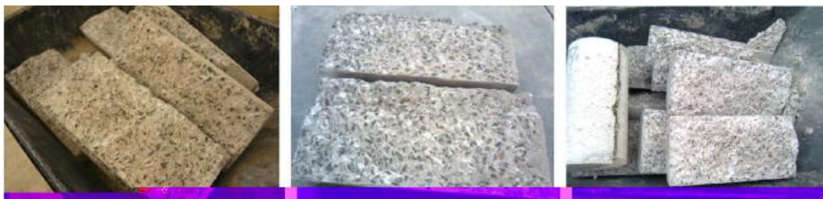
Fig. 4.12 Fracture surface of concrete cylinder specimen under tensile splitting load: (a) control concrete specimen, (b) 5% GRP waste powder admixed concrete, and (c) 15% GRP Waste powder.
