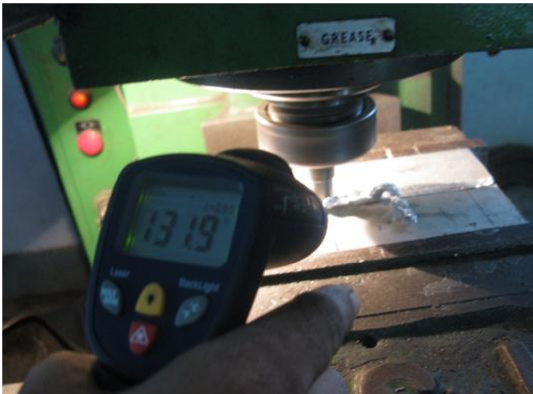
Figure 4.9: Measurement of temperature at mid point with the help of laser thermocouple.
