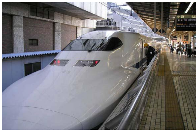
Figure 1.13: Japanese railway rolling stock fabricated from aluminum by FSW[20]
