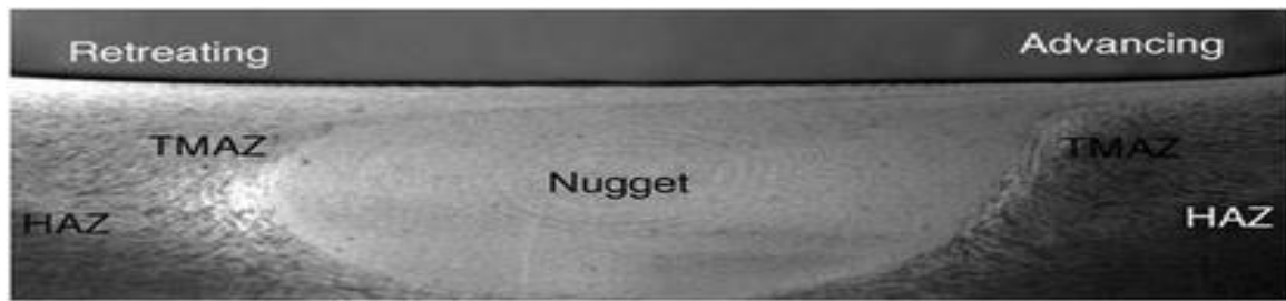
Figure 1.5: Transverse section of a friction stir weld showing different regions of the weld.
