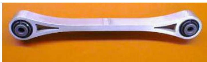
Figure 1.11: Automotive Link Arm Fabricated from Friction Stir Welding [8]
