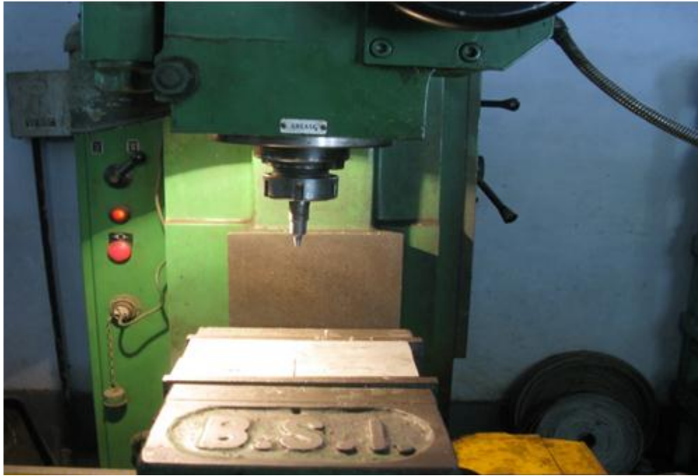
Figure 4.6: Plates are clamped firmly and tool is fixed.
