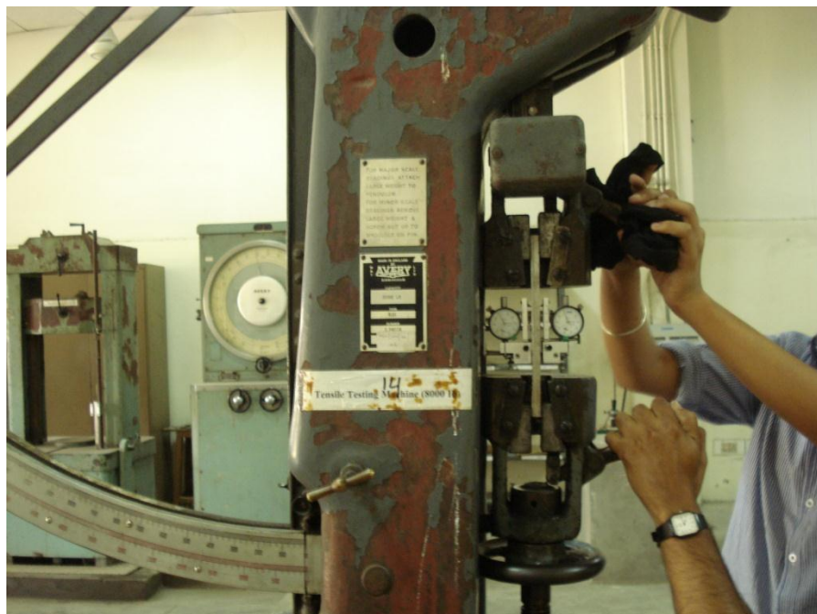
Figure4.14: Testing on Universal Testing machine with extensometer attached
