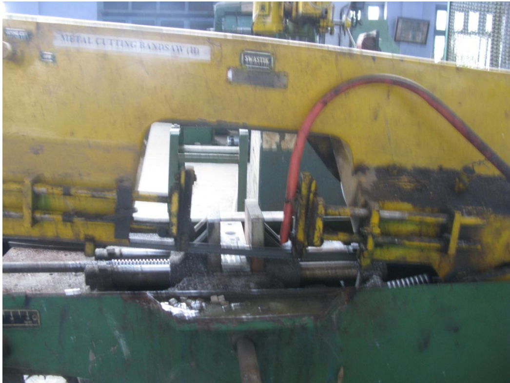
Figure 4.15 Samples preparation on band saw
