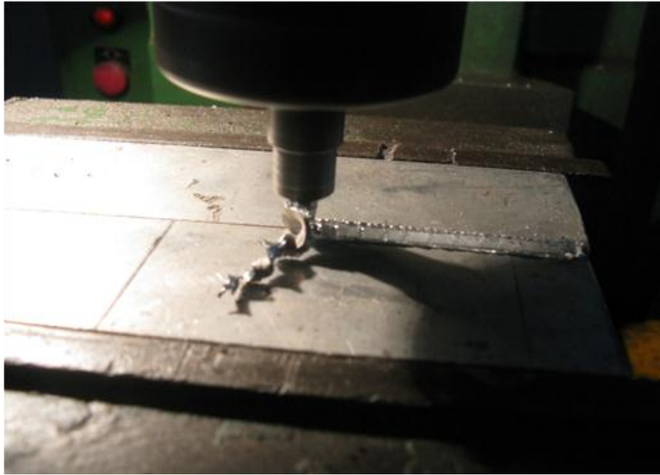
Figure 4.8 Tool is subsequently traversed along the joining line
