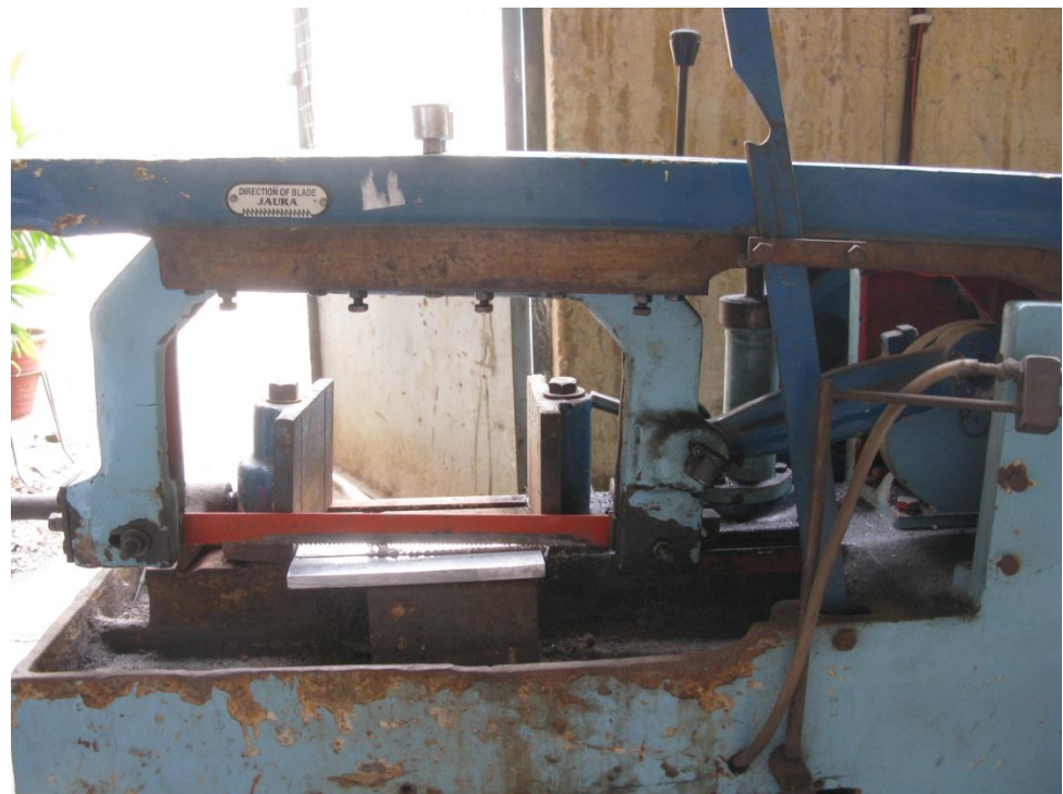
Figure 4.12: Sample preparation on power hacksaw
