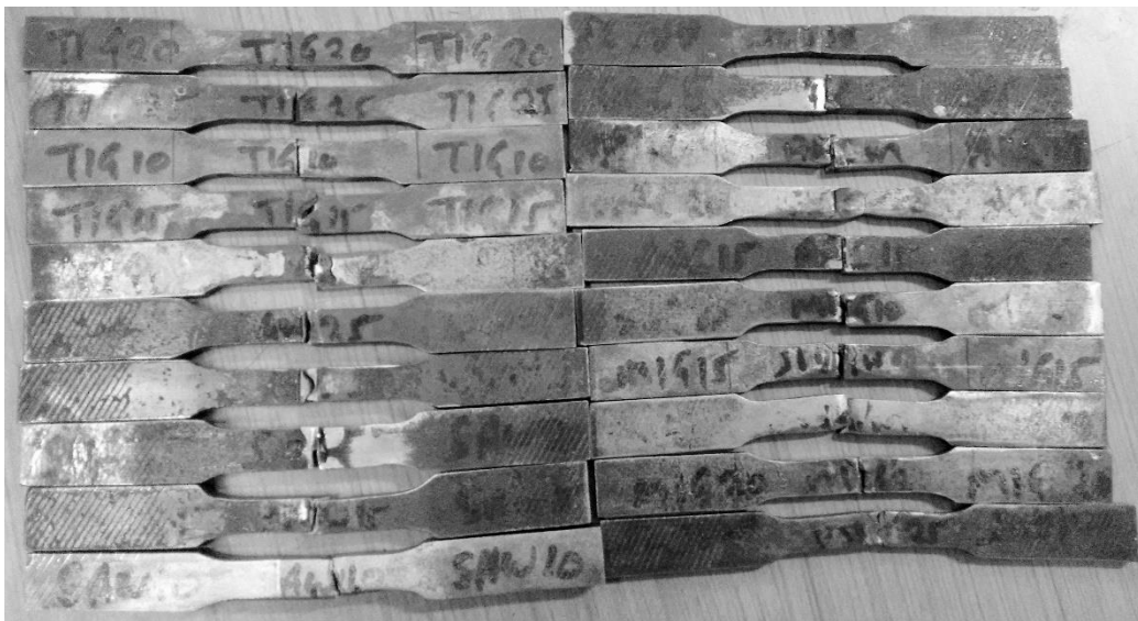
Figure 4.12: Tensile test specimens of medium carbon steel
