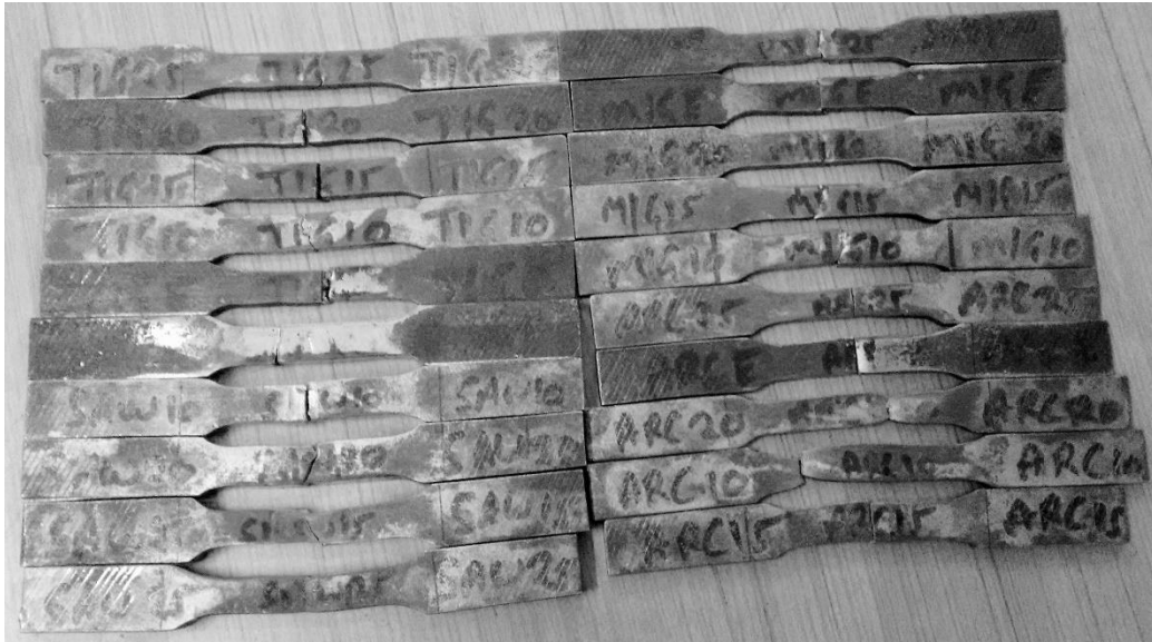
Figure 4.11: Tensile test specimens of low carbon steel
