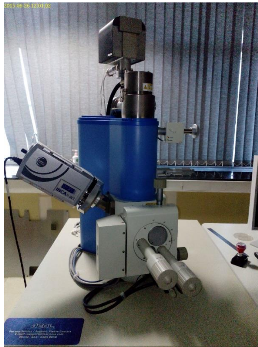
Figure 3.17: Scanning electron microscope + Energy dispersive spectroscopy (Courtesy; SAI Lab, Thapar University, Patiala)
