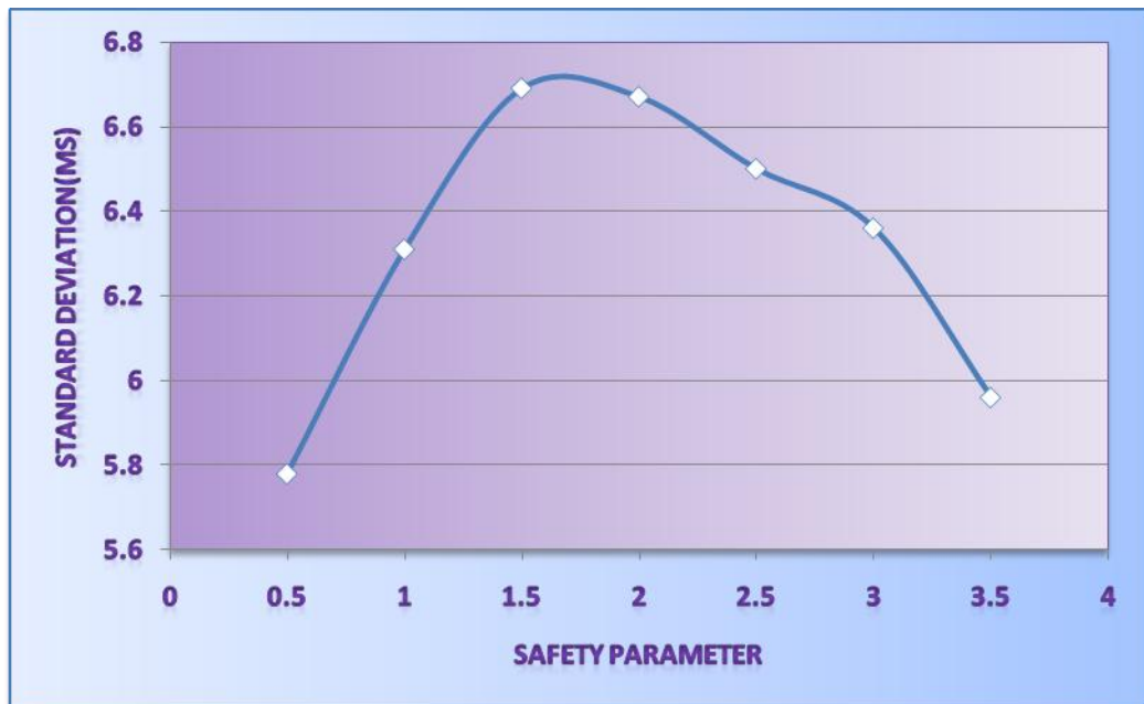
Fig 5.1 (d) Tradeoff between Safety Parameter and Standard Deviation for first case scenario
