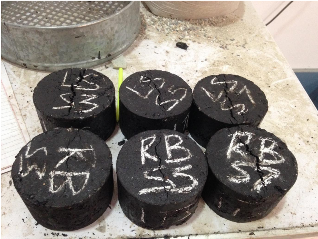
Figure 4.6: SBS modified samples after tensile failure
