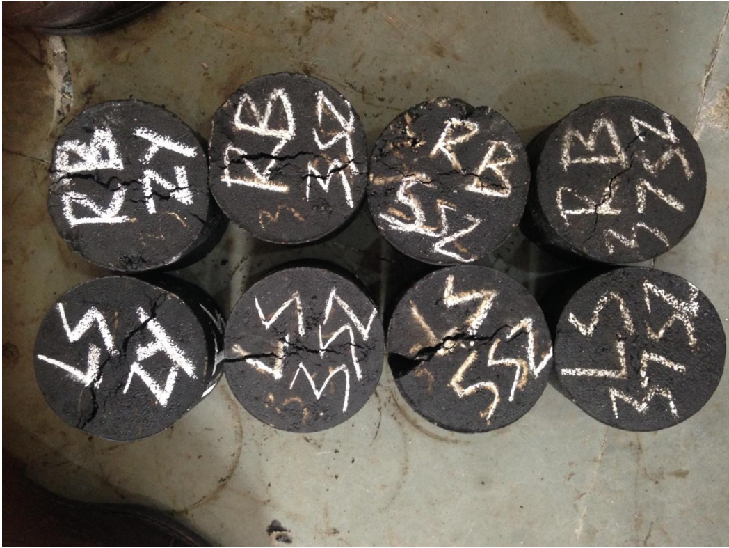
Figure 4.8: Zycotherm modified bitumen samples after tensile failure
