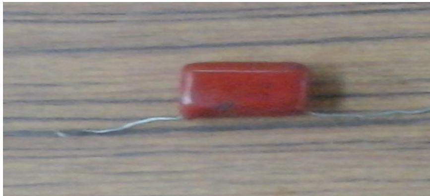
Figure 3.7: Capacitor of 1 microfarad
