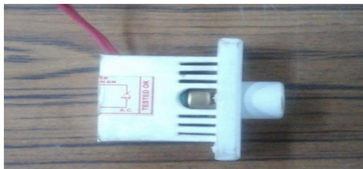
Figure 3.8: Volume type regulator
