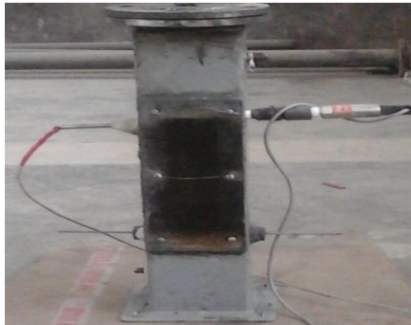
Figure 3.4: Explosion Container used in experiment
