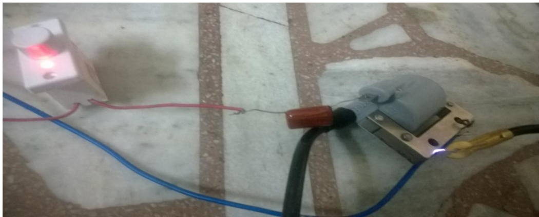
Figure 3.6: spark produced by ignition coil
