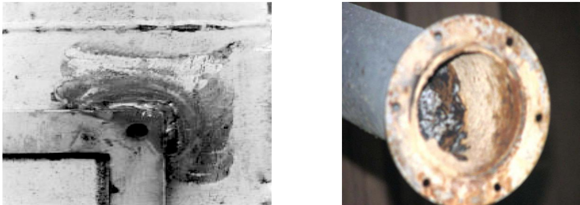
Figure 2.1: Burning at the welded joint and dust explosion in pipe [2]
