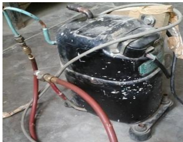
Figure 3.14: Compressor and Vacuum pump
