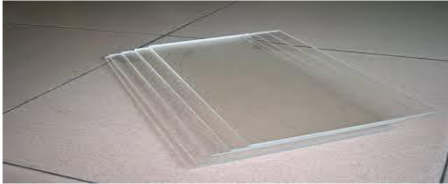
Figure 3.5: Sight glass (Acrylic sheet)
