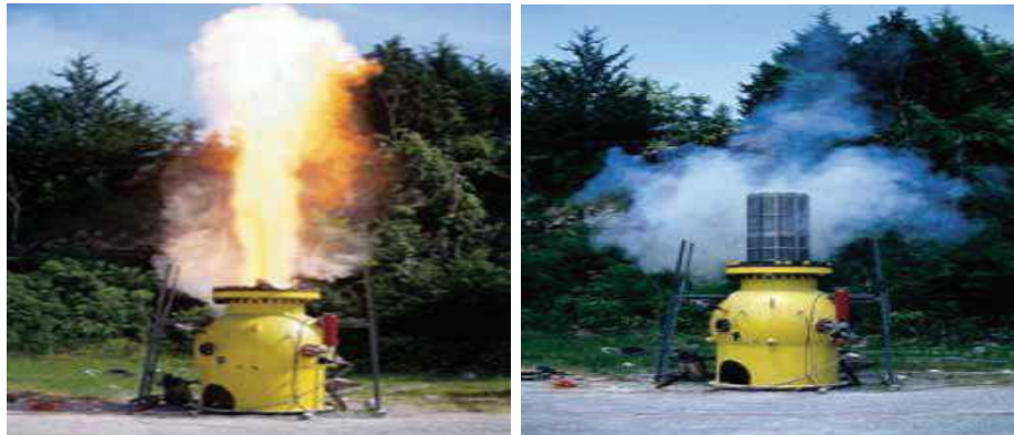
Figure2.4: Explosion before and after using flameless venting [13]
