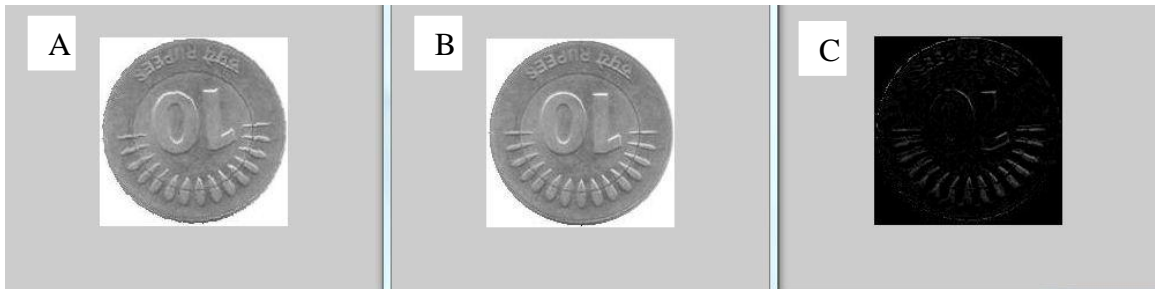
Figure 1.7: Example of image subtraction (A) image 1 (B) image 2 (C) result image
