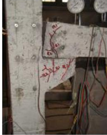
Fig. 2.5. Failed J-bolt connection
