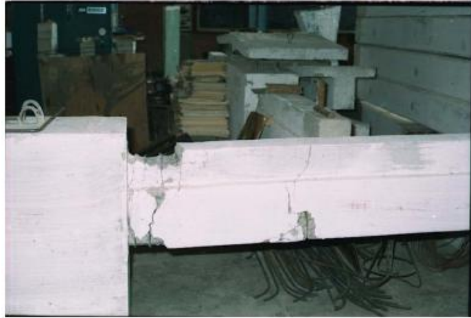
Fig. 2.38. Test specimens PM1 at the end of the test and damage condition.
