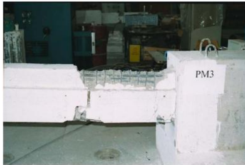
Fig. 2.40 Test specimens PM3 at the end of the test and damage condition.
