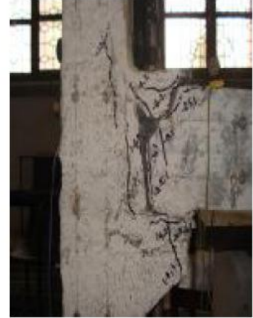
Fig. 2.6. Failed cleat angle connection
