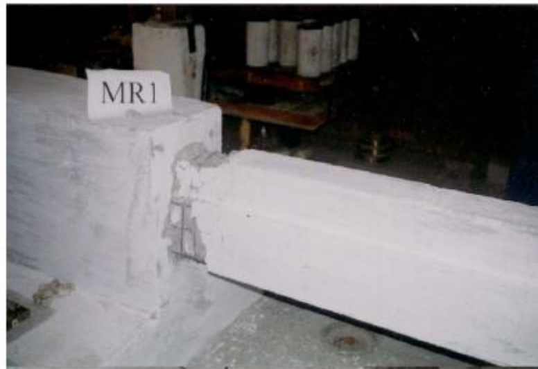
Fig. 2.36. Test specimens MR1 at the end of the test and damage condition.
