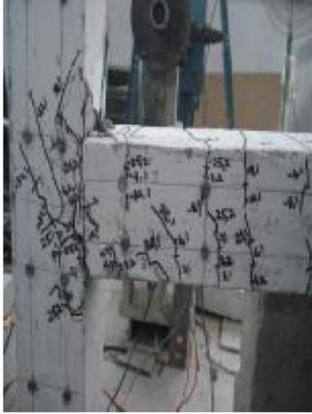
Fig. 2.4 Failed monolithic specimen
