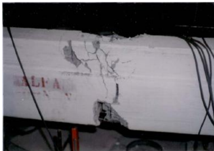
Fig. 2.39 Test specimens PM2 at the end of the test and damage condition.
