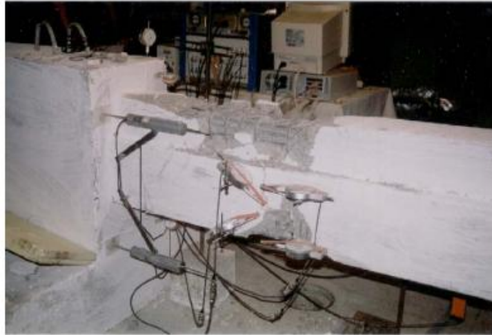
Fig. 2.37. Test specimens PO1 at the end of the test and damage condition.
