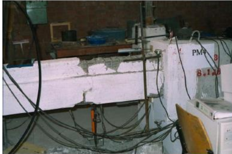
Fig. 2.41. Test specimens PM4 at the end of the test and damage condition.
