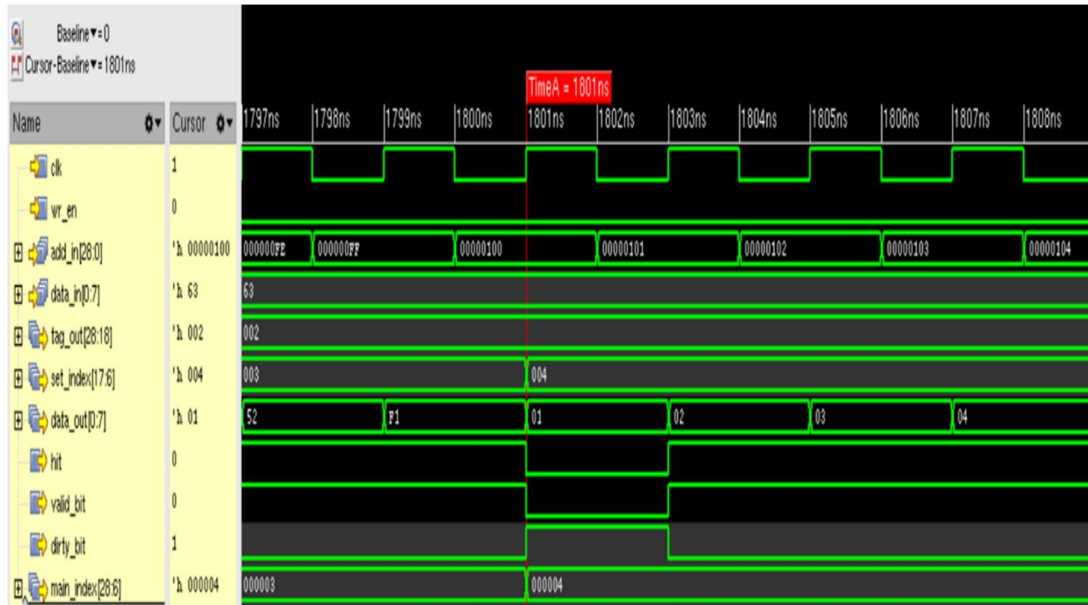
Figure 7.3 Cache Miss in a Two-Way Mapping.
