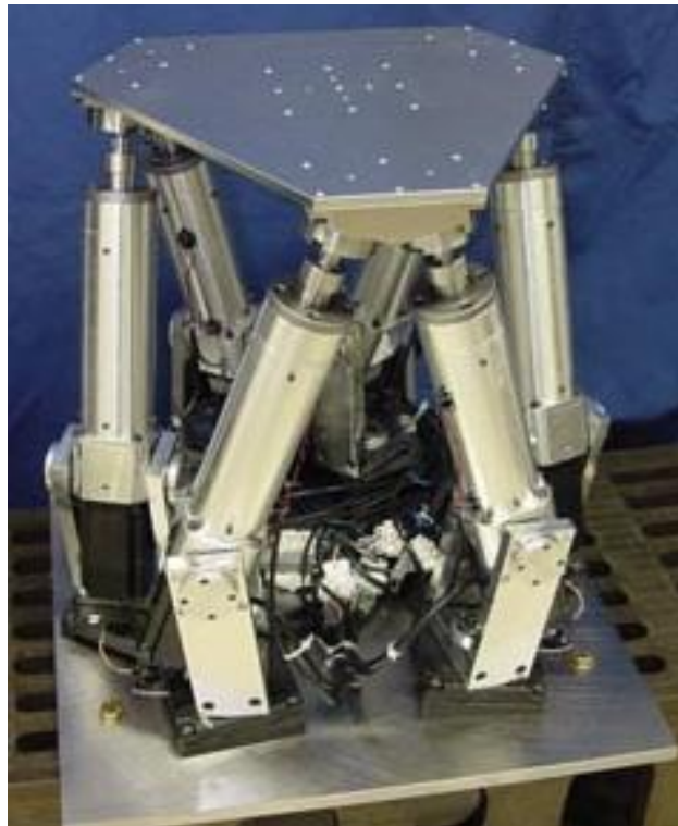
Fig. 1.3: A parallel-serial hybrid manipulator [G5].
