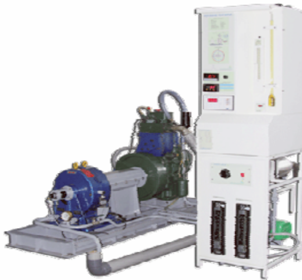
Fig.5.1 VARIABLE COMPRESSION RATIO ENGINE SET UP [36]
