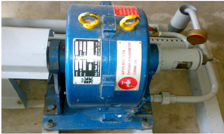
Fig 2.3 DYNAMOMETER USED IN VARIABLE COMPRESSION RATIO TEST RIG USED TO VARY LOAD [35]
