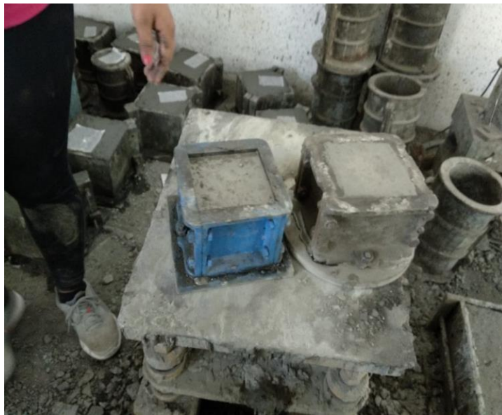
Figure 5.6: Compaction of concrete on Table Vibrator
