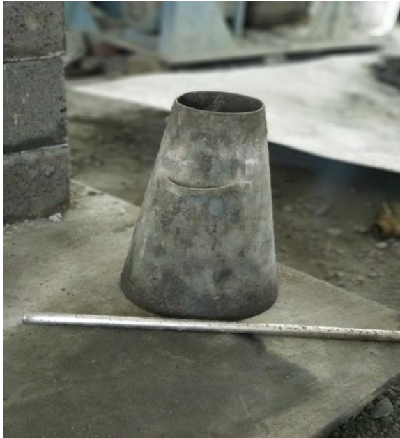
Figure 5.7: Slump test apparatus- slump cone and tamping rod
