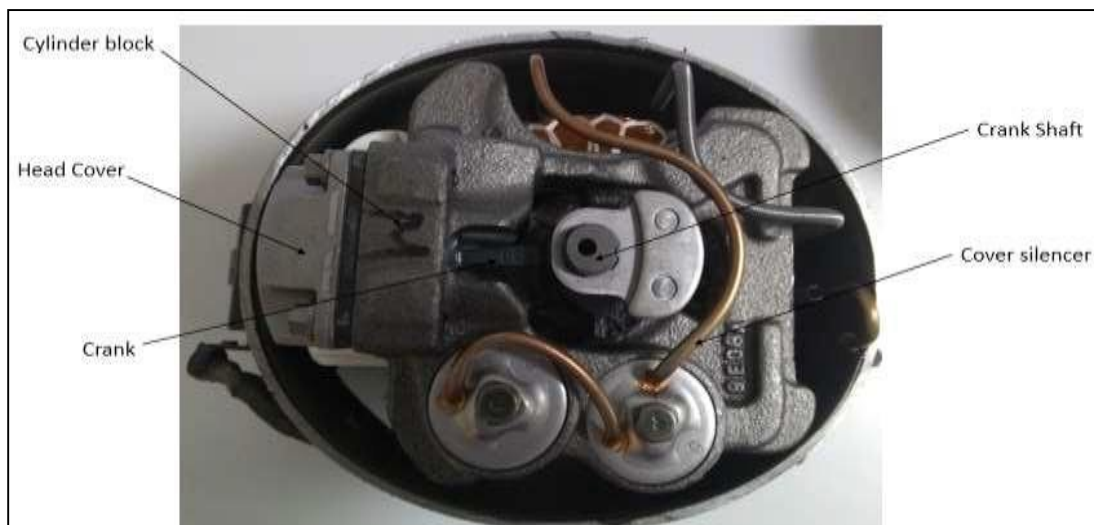
Fig. 13: Assembly of hermetic compressor (top view) [LG. electronics India]
