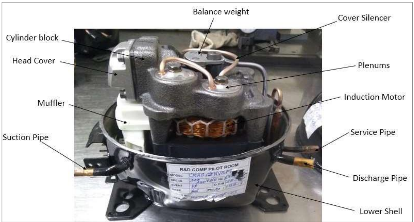
Fig. 14: Assembly of hermetic compressor (side view) [LG. electronics India]
