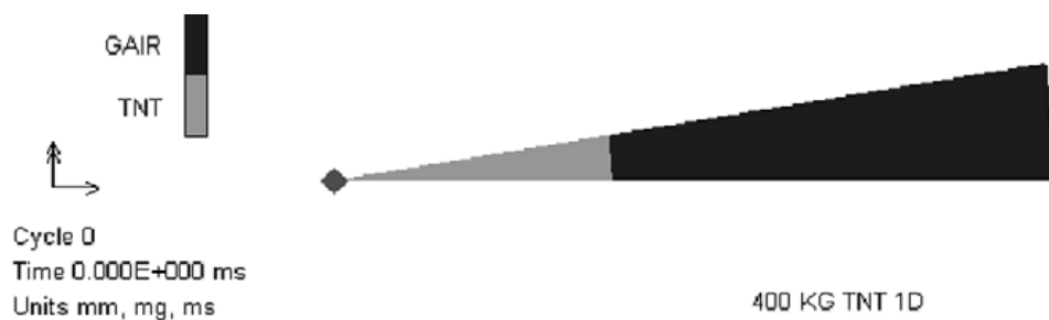
Fig. 3.2. Mesh used for the generation of the explosion (400 kg TNT)
