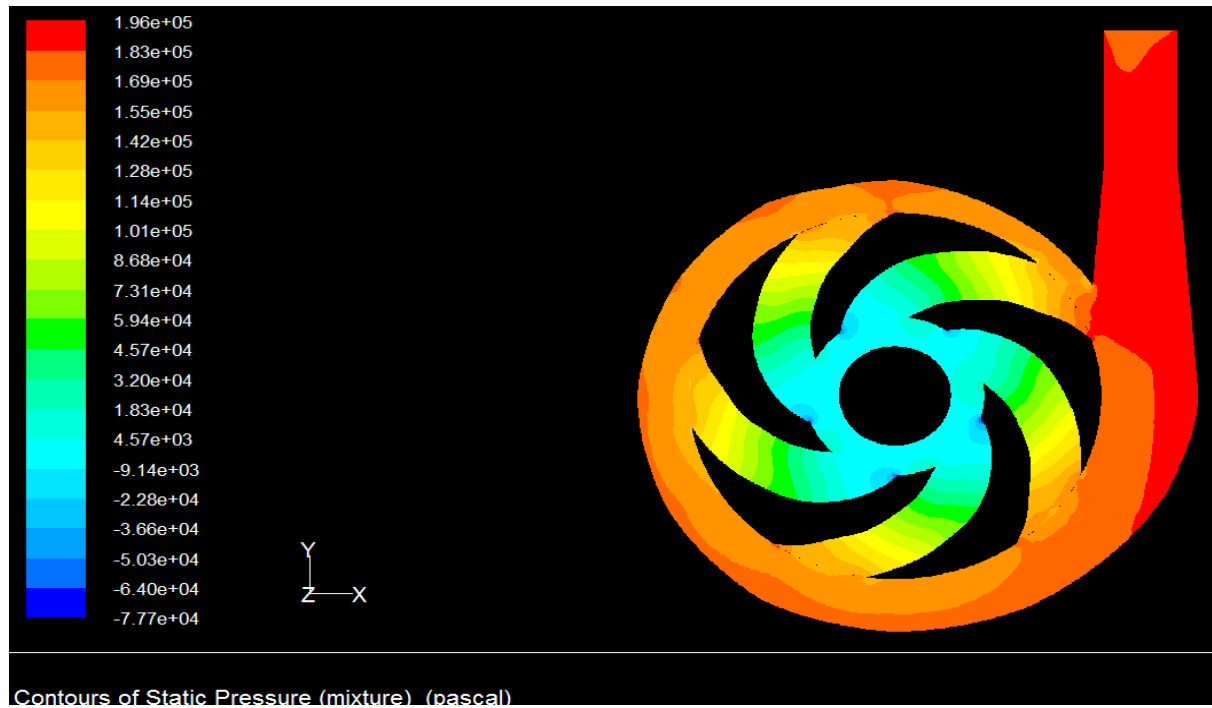
Figure 3.5: Static Pressure contour for concentration of Bottom Ash (20% by weight) at 1450 rpm and ( Q/Q_{BEP}=1 )
