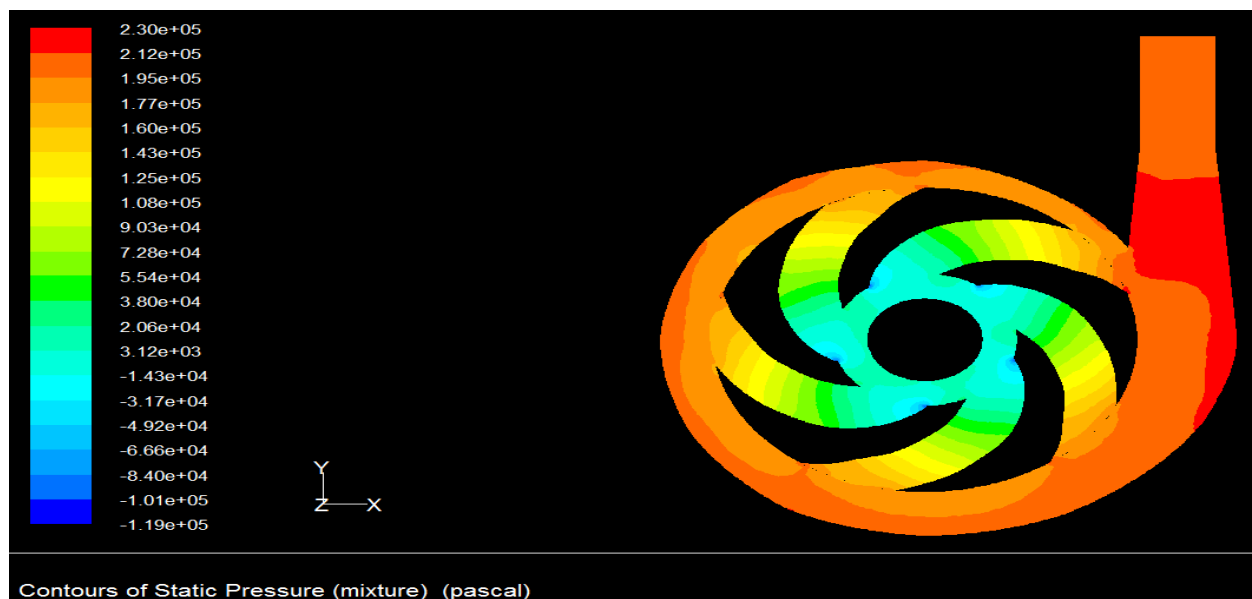
Figure 3.6: Static Pressure contour for concentration of Bottom Ash (50% by weight) at 1450 rpm and ( Q/Q_{BEP}=1 )
