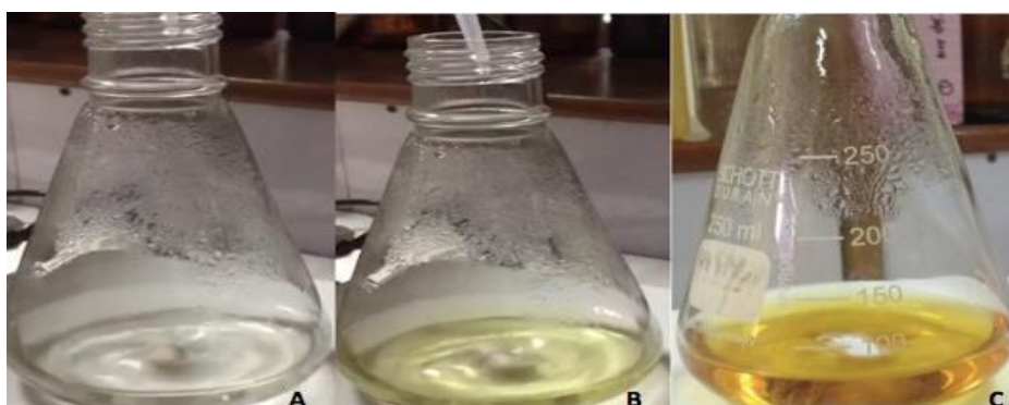
Fig 16 :- Synthesis of chitosan stabilized silver nanoparticles A) chitosan + \text{AgNO}_3 B) addition of \text{NaBH}_4 C) Ch-Ag NPs
