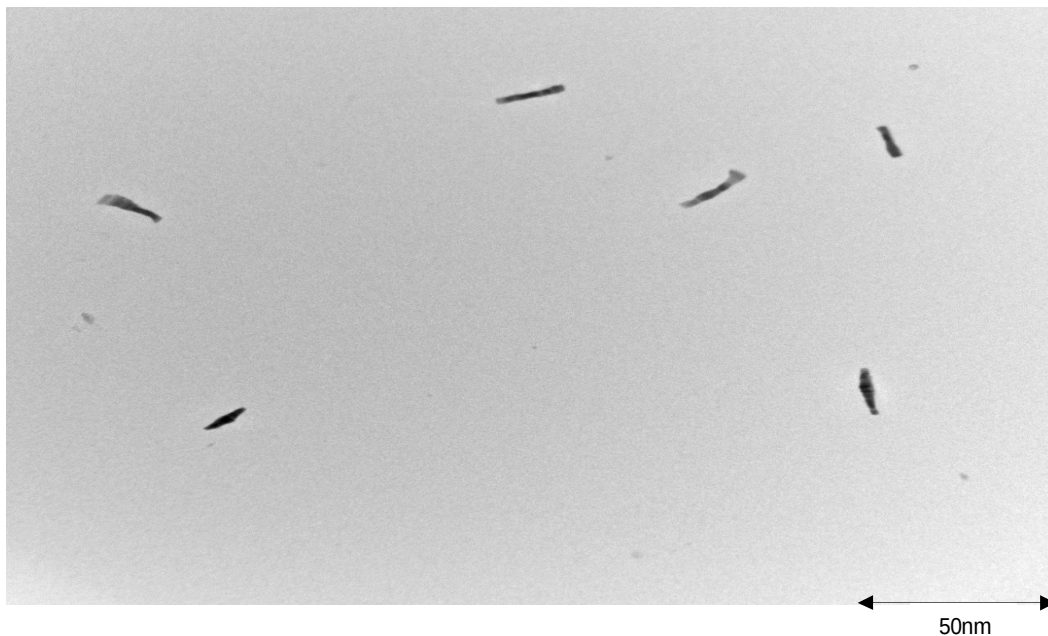
Fig 4.19 : TEM image of \text{Mn}_3\text{O}_4 - \text{La}(\text{OH})_3 nanocomposite.
