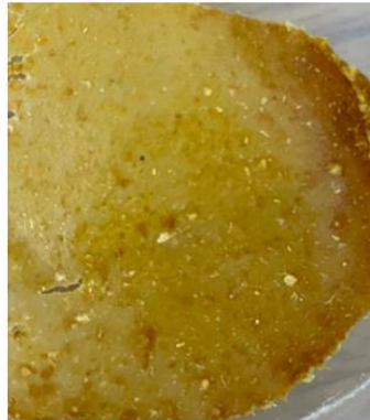
Membrane prepared from orange peel powder, without utilization of glycerol as plasticizer
