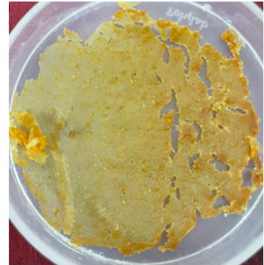
Membrane prepared from orange peel powder, without utilization of sorbitol as plasticizer
