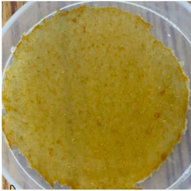
Membrane prepared from orange peel powder, without utilization of any plasticizer
