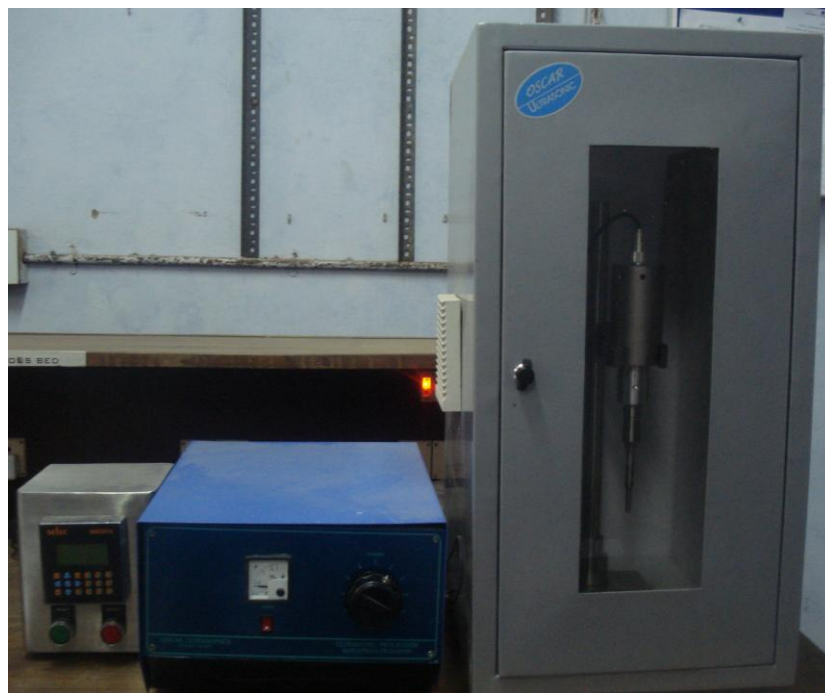
Fig 4.5: Oscar Ultra Sonicator (Probe Type)
