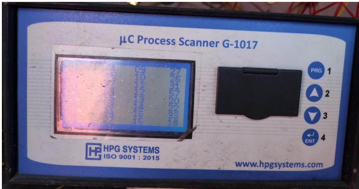
Fig. 3.14 Temperature data logger
