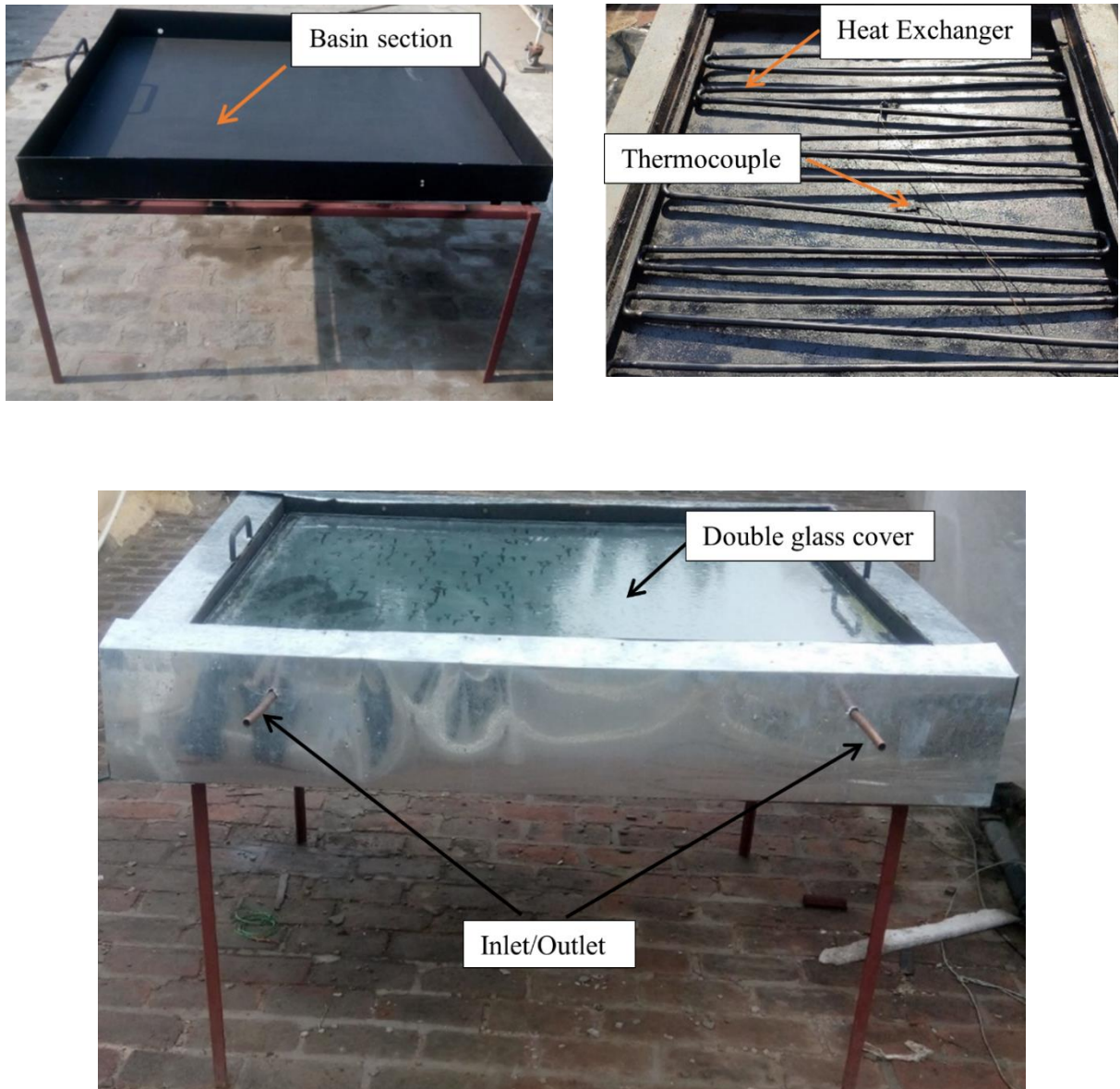
Fig. 3.4 Nanofluid-based volumetric absorption solar collector.
