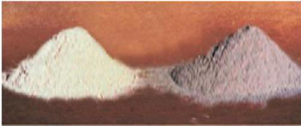
Figure 1.3 : Typical ash colours (Class “F” & “C” fly ash) (J.Alam and M.N Akhtar 2011)
