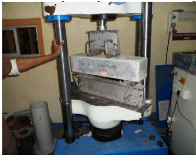
Figure 2.7 : Flexural strength test (Solanki & Pitroda, 2013)
