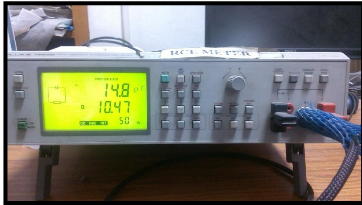
Fig. 2.9: View of LCR bridge used for dielectric analysis.
