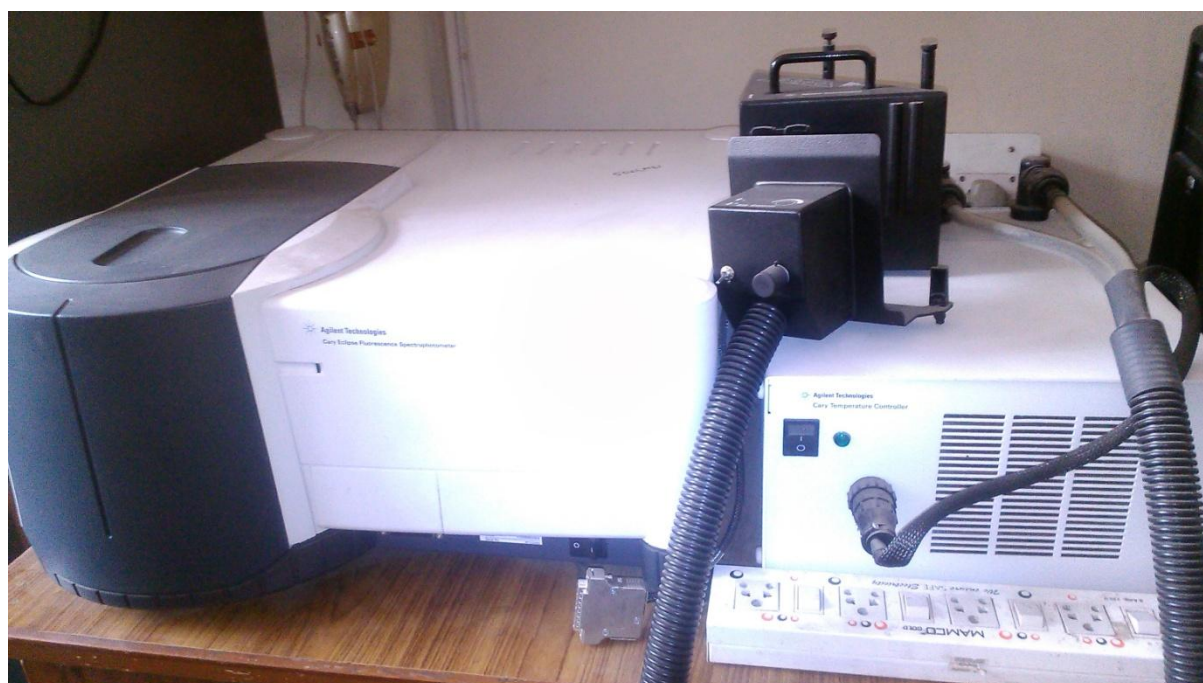
Fig. 2.6: View of Fluorescence Spectrophotometer used for sample analysis.
