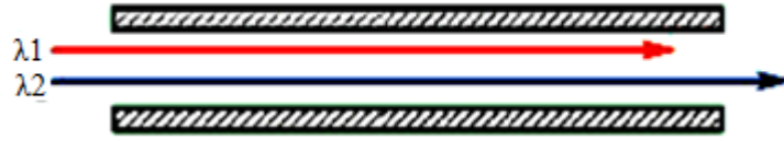
Figure 2.6: Waveguide dispersion in step index fiber
