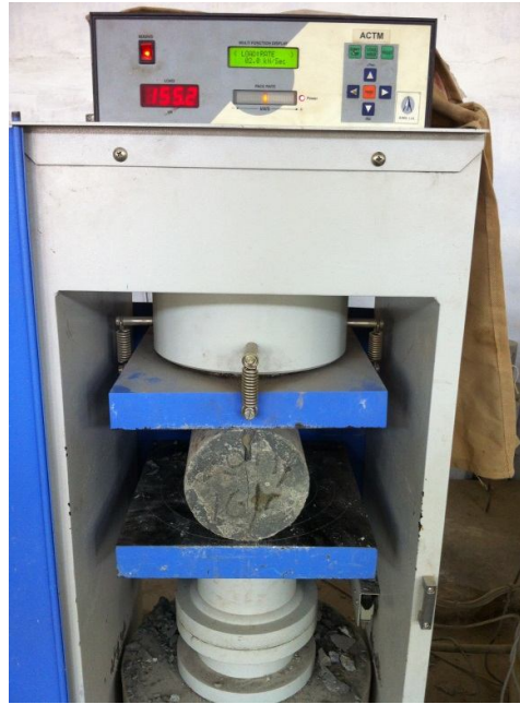
Fig 3.3: Cylinder specimen subjected to split tensile strength
