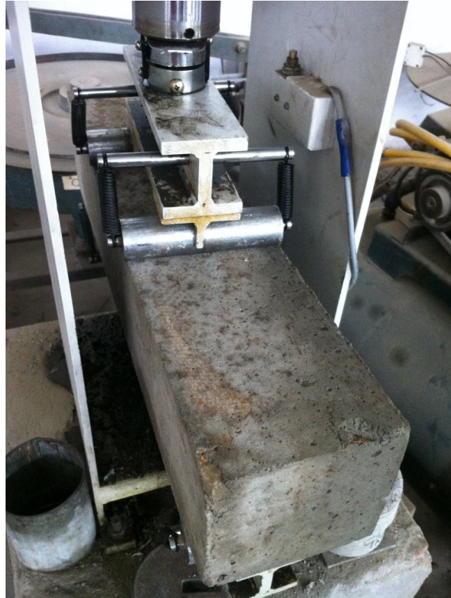
Fig 3.4 Beam specimen subjected to two point loading
