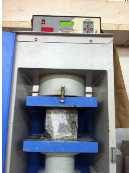
Fig 3.2 Cube specimen subjected to compression
