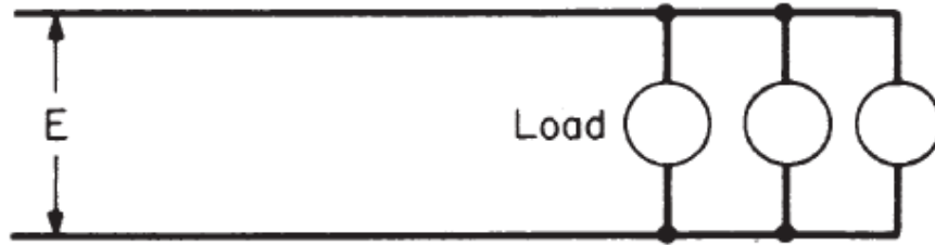
Figure 1.3 AC single-phase two- wire system.
