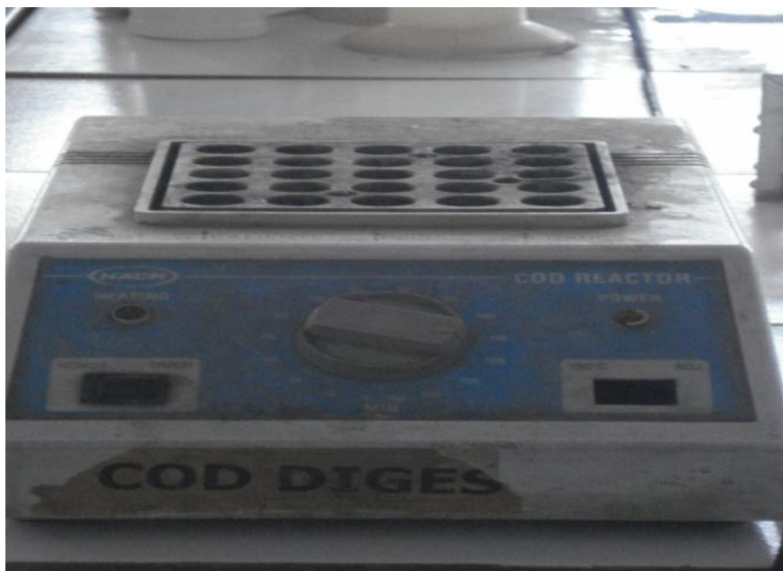
Fig-3.4 COD digester
