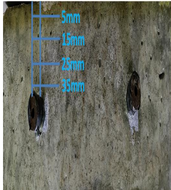
Figure 4-11 Drilling positions From Top. Figure 4-12 Drilling position with depth.
