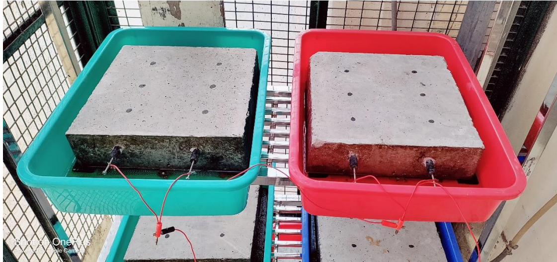
Figure 4-8 Experimental Setup of BIEM
