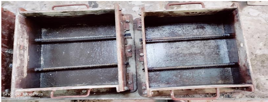
Figure 4-3 Moulds prepared for casting.
