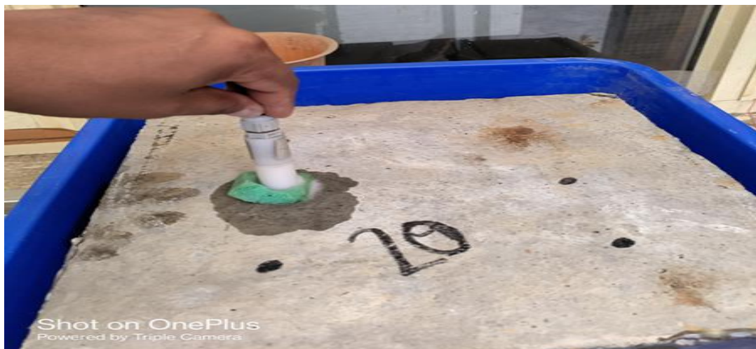
Figure 4-9 Measurement of HCP using WE
