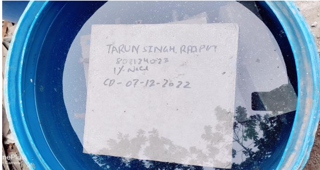
Figure 4-7 Curing of Specimens in NaCl water.
