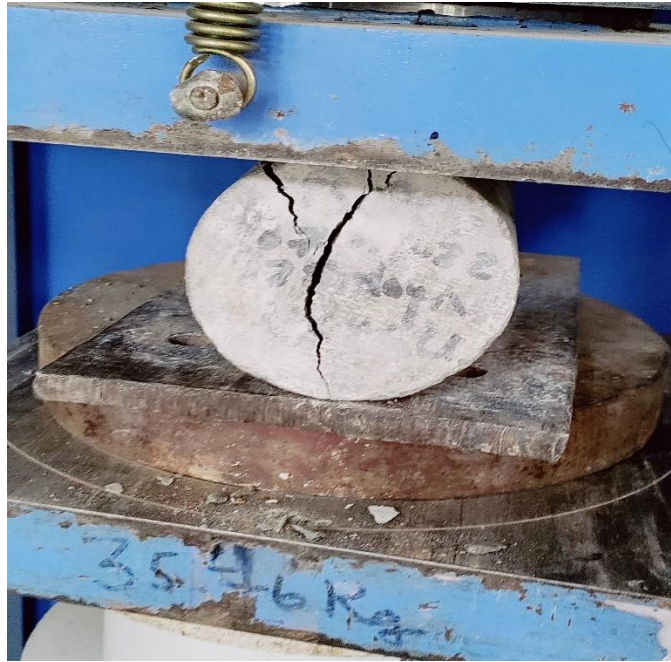
Figure 4-18 Split Tensile Testing
