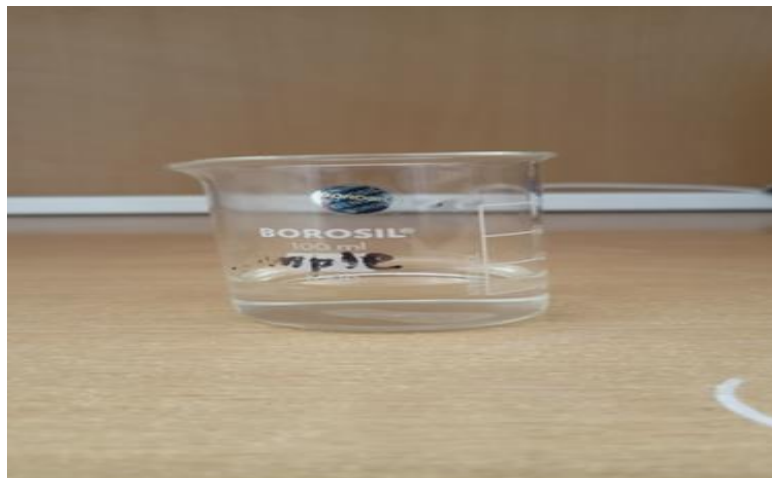
Figure 4-13 Prepared sample for chloride testing.
