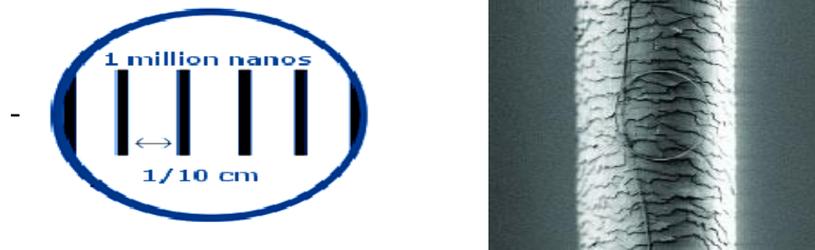
Fig. 1.1 Comparison of nm scale with cm scale and a micrograph shows a nanowire curled into a loop in front of a human hair.
