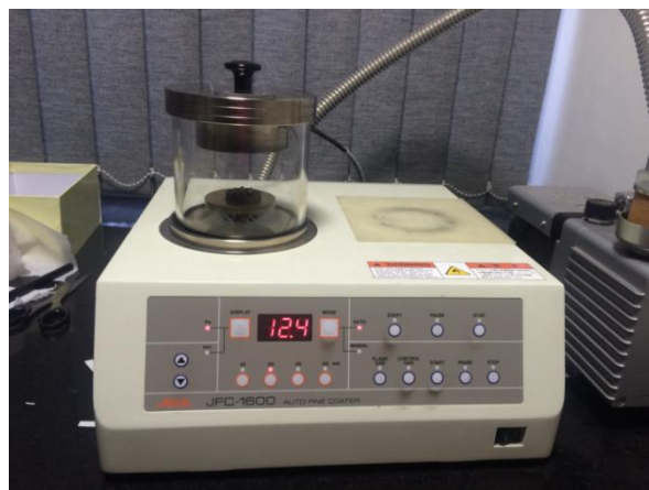
Figure 4.21: Deposition system for coating insulating SEM samples
