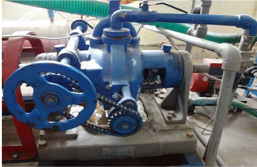
Figure 4.10 Hydraulic dynamometer used to load the engine
