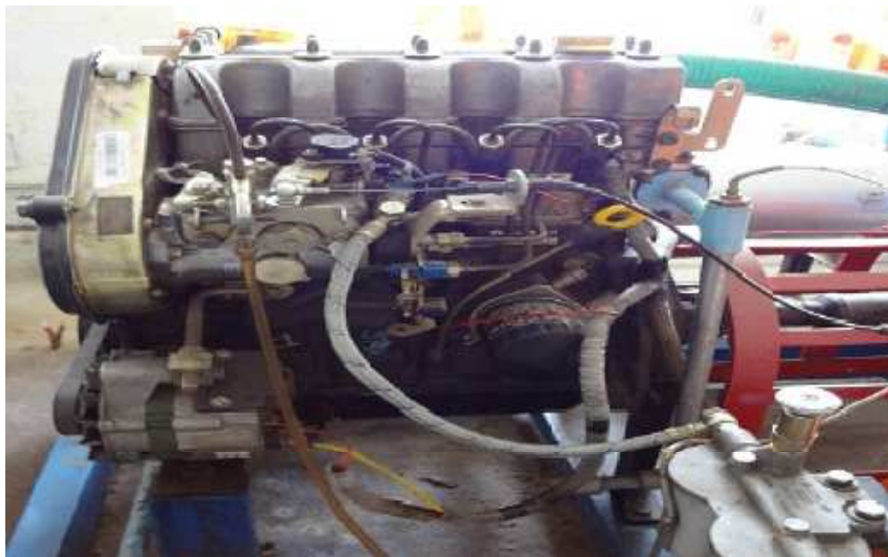
Figure 4.9 Tata make 1400cc, 4-cylinder, 4-stroke, DI Engine
