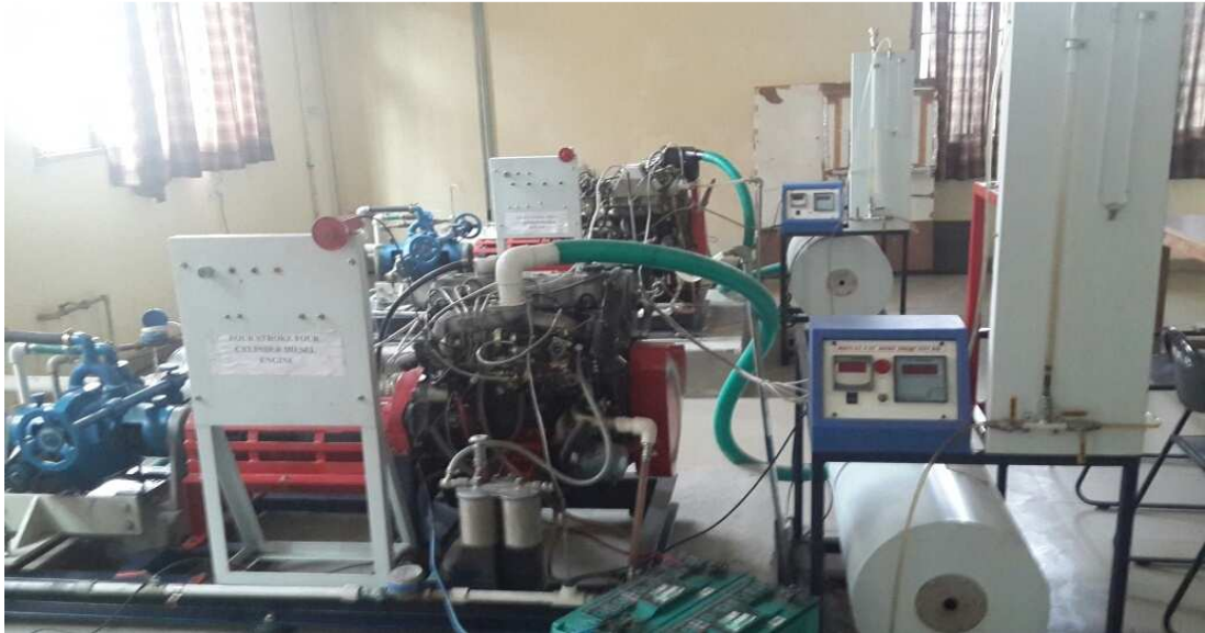
Figure 4.8 Test rig of 4-cylinder,4-stroke diesel Engine
