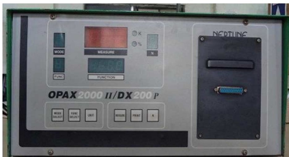
Figure 4.14 Smoke Meter to measure smoke opacity
