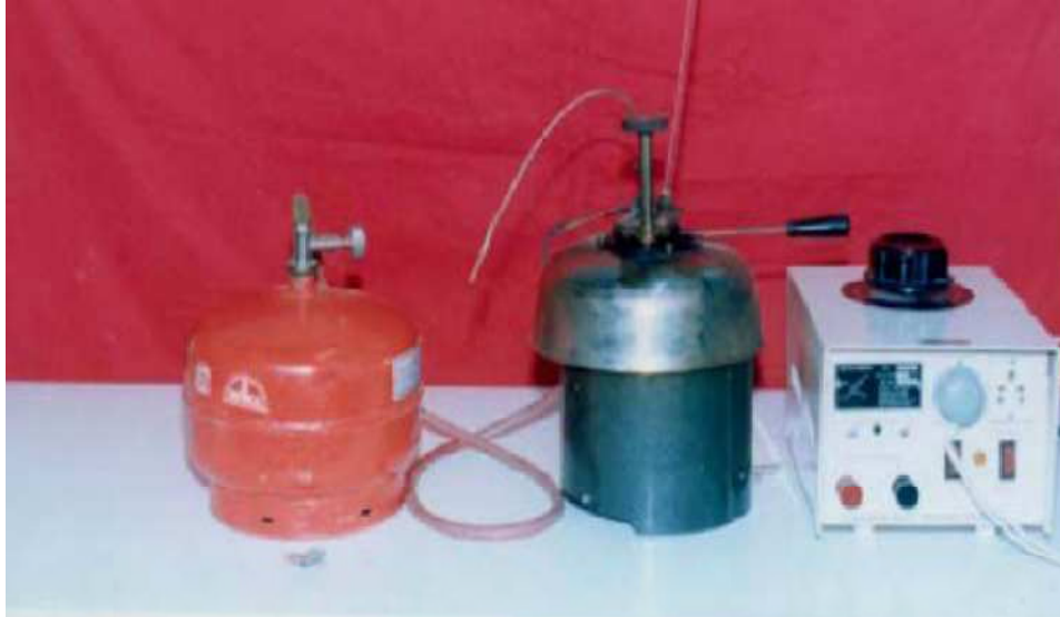
Figure 4.7 Flash and fire point measurement using Pensky martin apparatus
