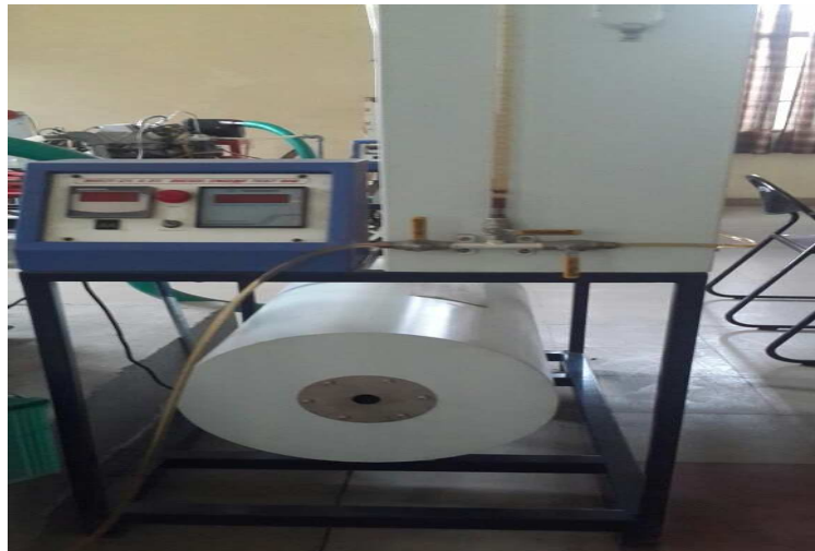
Figure 4.12 Fuel and Air consumption measuring arrangement
