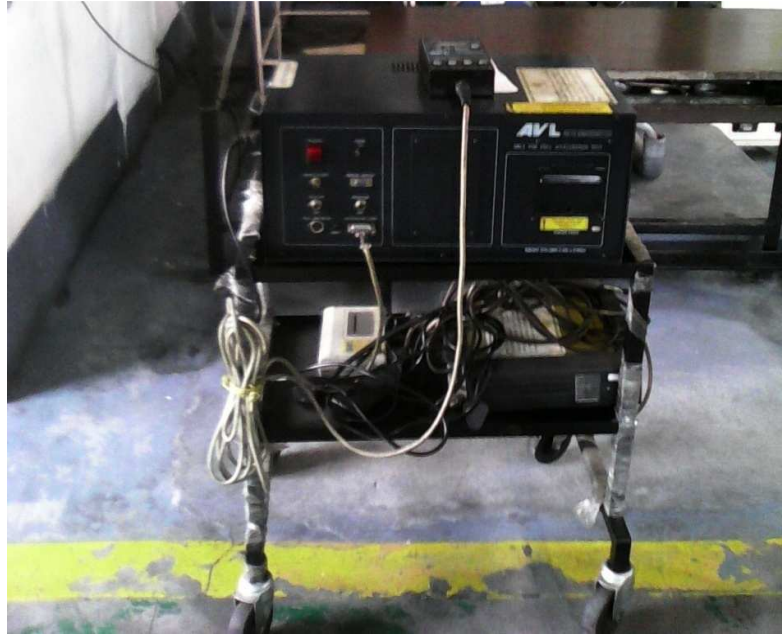
Figure 4.15(a) Control panel view of AVL flue gas analyzer
