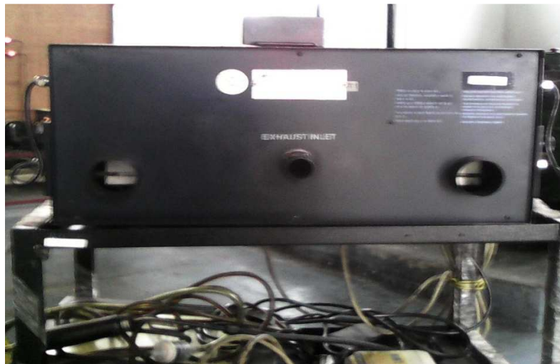
Figure 4.15(b) Exhaust inlet of AVL flue gas analyzer.
