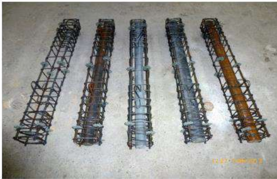
Fig.2.5 (a) View of the column Reinforcement consisting of different types of cylindrical steel and UHSC core [Hudoba and Mikus, 2013]
