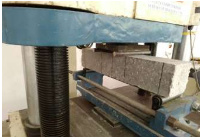
Fig. 4.9: Beam under UTM
