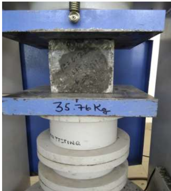
Fig.3.5: Automatic Compression Testing Machine (5000 KN Capacity)
