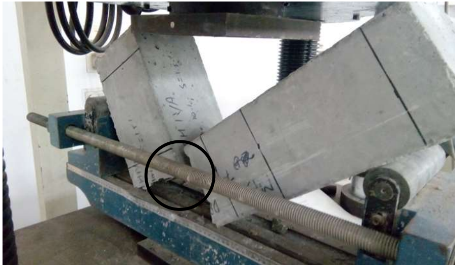
Fig. 4.15 Failure pattern of beam
