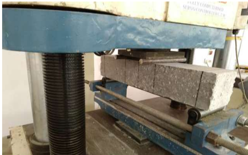
Fig.3.7: Beam Testing Arrangement
