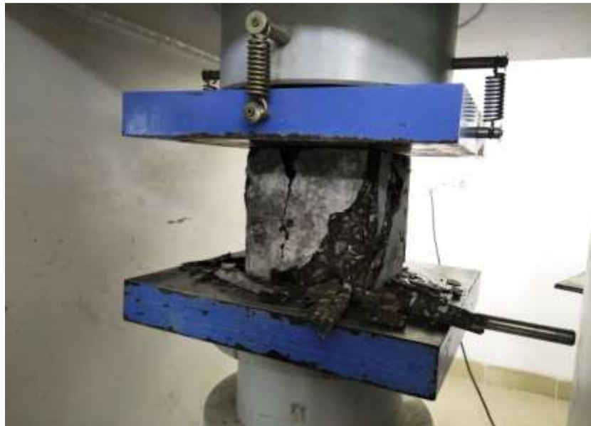
Fig.4.1: Cube under compression in Automatic Compression Testing Machine (ACTM)
