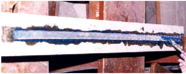
Fig. 1. 20 mm wide E-glass sheet bonded to plain concrete beam.
