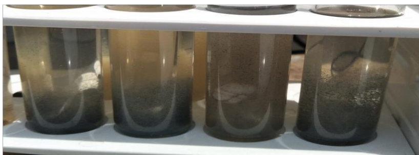
Fig.13: Changes in UV absorption ( \lambda_{\text{max}} 400 nm) spectra/color of tie dye due to its photo degradation (a) \text{TiO}_2 and (b) \text{GO-TiO}_2 under sunlight irradiation for 120 minutes.
