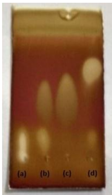
Fig. 6: Thin Layer Chromatography analysis of (a) glycerol ( R_f = 0.32 ), (b) reaction mixture ( R_f = 0.32 ), ( R_f = 0.56 ) (c) TEGDME ( R_f = 0.56 ), (d) Glycerol carbonate ( R_f = 0.63 )
