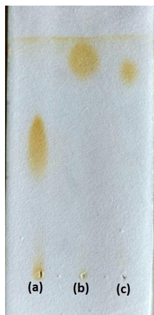
Fig.3: TLC analysis of (a) cotton seed oil ( R_f = 0.63 ), (b) cotton seed oil derived FAME ( R_f = 0.9 ), (c) methyl oleate standard ( R_f = 0.9 ).
