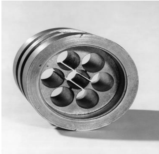
Figure 1.1 Anode block Cavity- Magnetron discovered by John Randall and Harry Boot [1]
