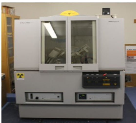
Fig 3.4.1(b) Experimental set up of X-ray diffractometer ("PANalytical X'Pert-Pro XRD)
