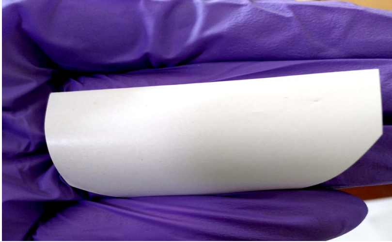
Fig 3.3 BCZT/PVDF composite film after drying at 80°C and peeled off from the glass plate
