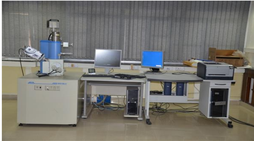
Fig 3.4.3 Experimental set up of scanning electron microscope (SEM)
