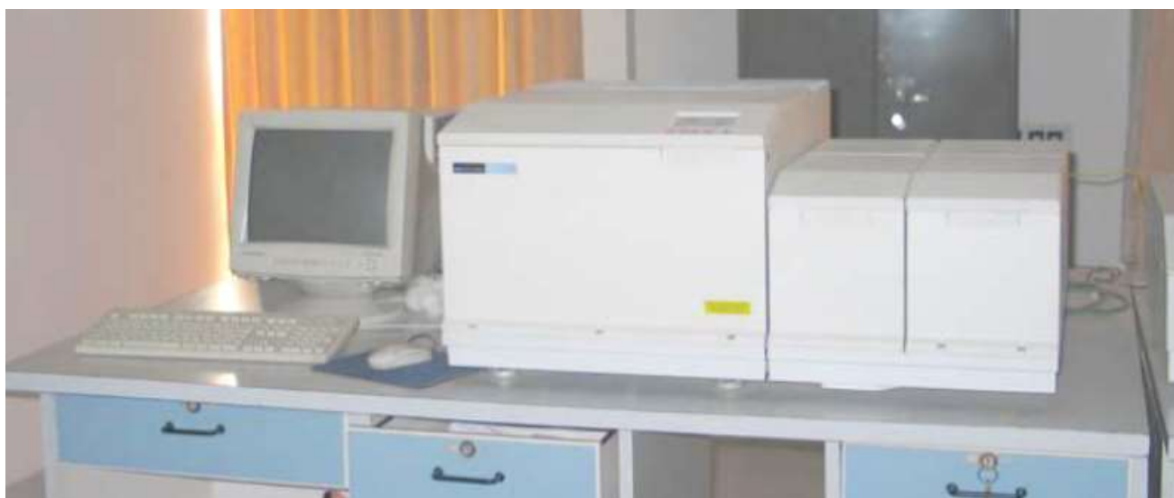
Fig 3.4.2(b) Experimental set up of FTIR spectrometer
