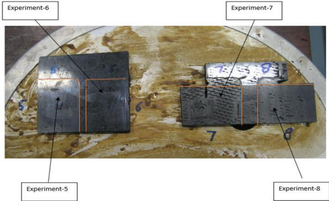
Fig. 3. 9: C/SiC of material density 2.18 \text{ g/cm}^3 after RUM
