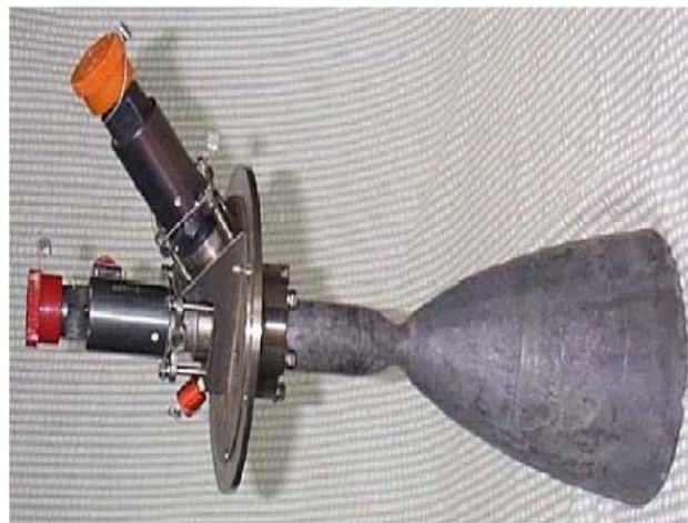
Fig. 1. 6: 150 N C/SiC thruster (developed and tested by China) (7)
