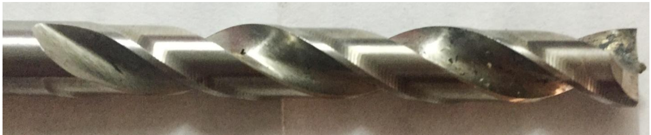
Figure 3.6 HSS brad point drill(8mm diameter)
