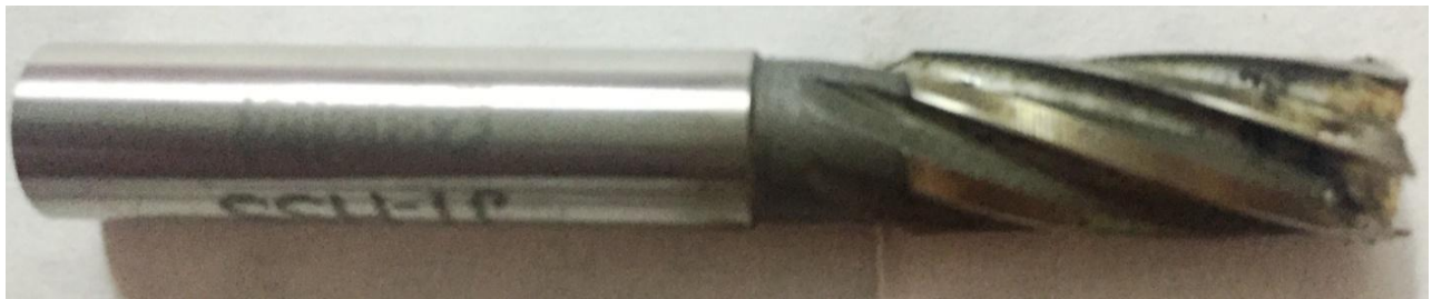
Figure 3.7 Six Flute HSS end mill(8mm diameter)
