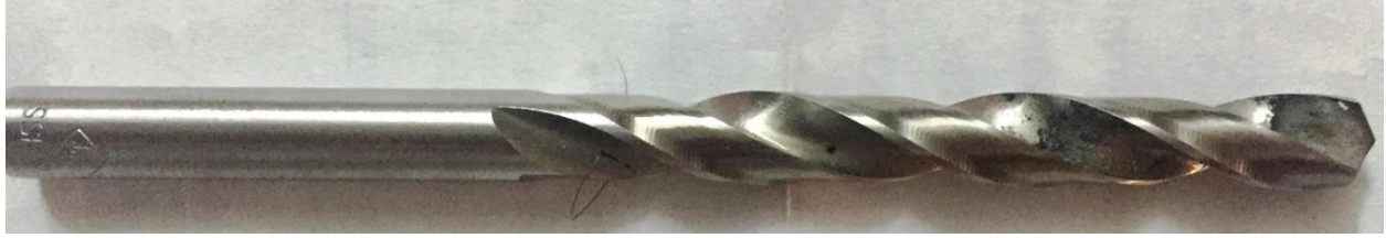
Figure 3.5 HSS twist drill(8mm diameter)
