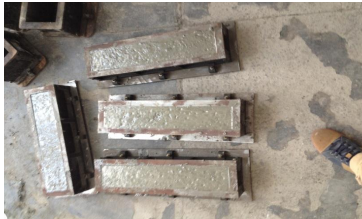
Fig. 3.14: Beams for flexural strength test
