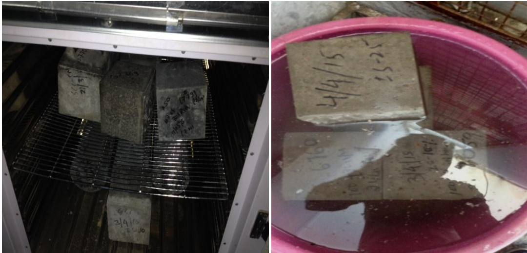
Fig. 3.16: Specimens in oven for drying and in water for absorption
