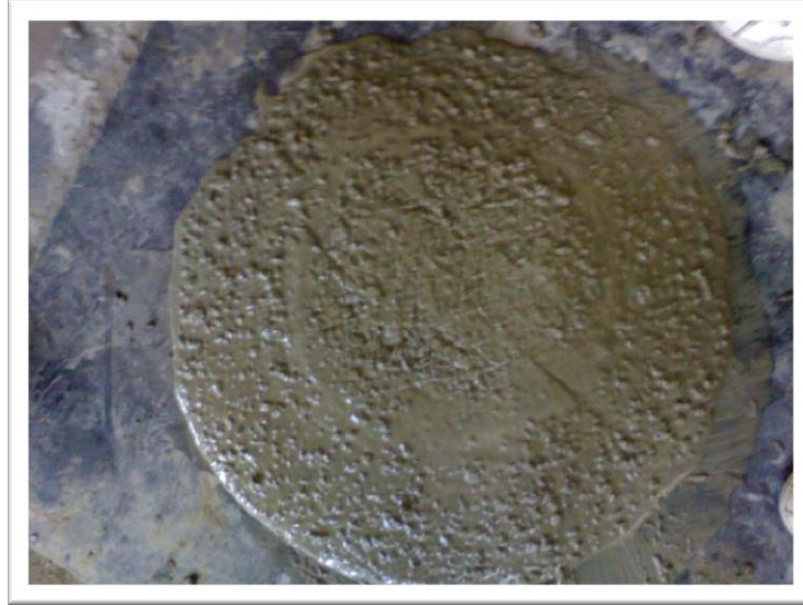
Fig 4.2: Slump flow during testing
