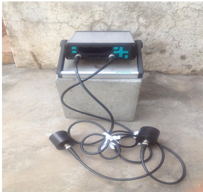
Fig. 3.19: Ultra-sonic pulse velocity set up
