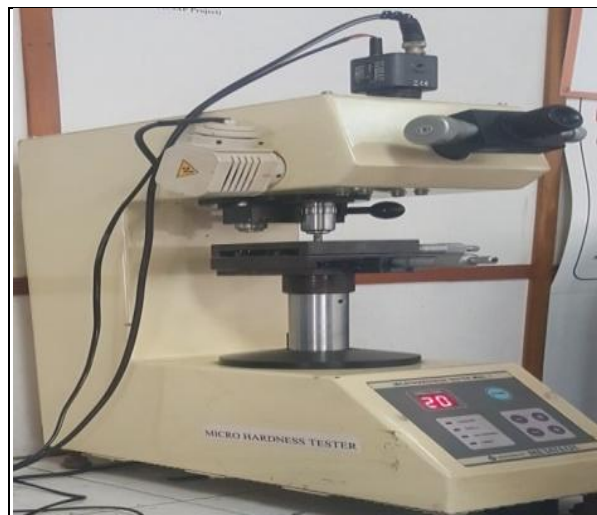
Figure 3.5 Micro-hardness tester [Photo Courtesy: Thapar university campus, Patiala]
