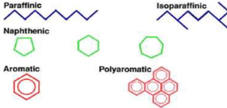
Figure 2.1: Basic hydrocarbon structures of Mineral oil
