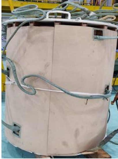
Figure 5.6: Continuous double disc winding
