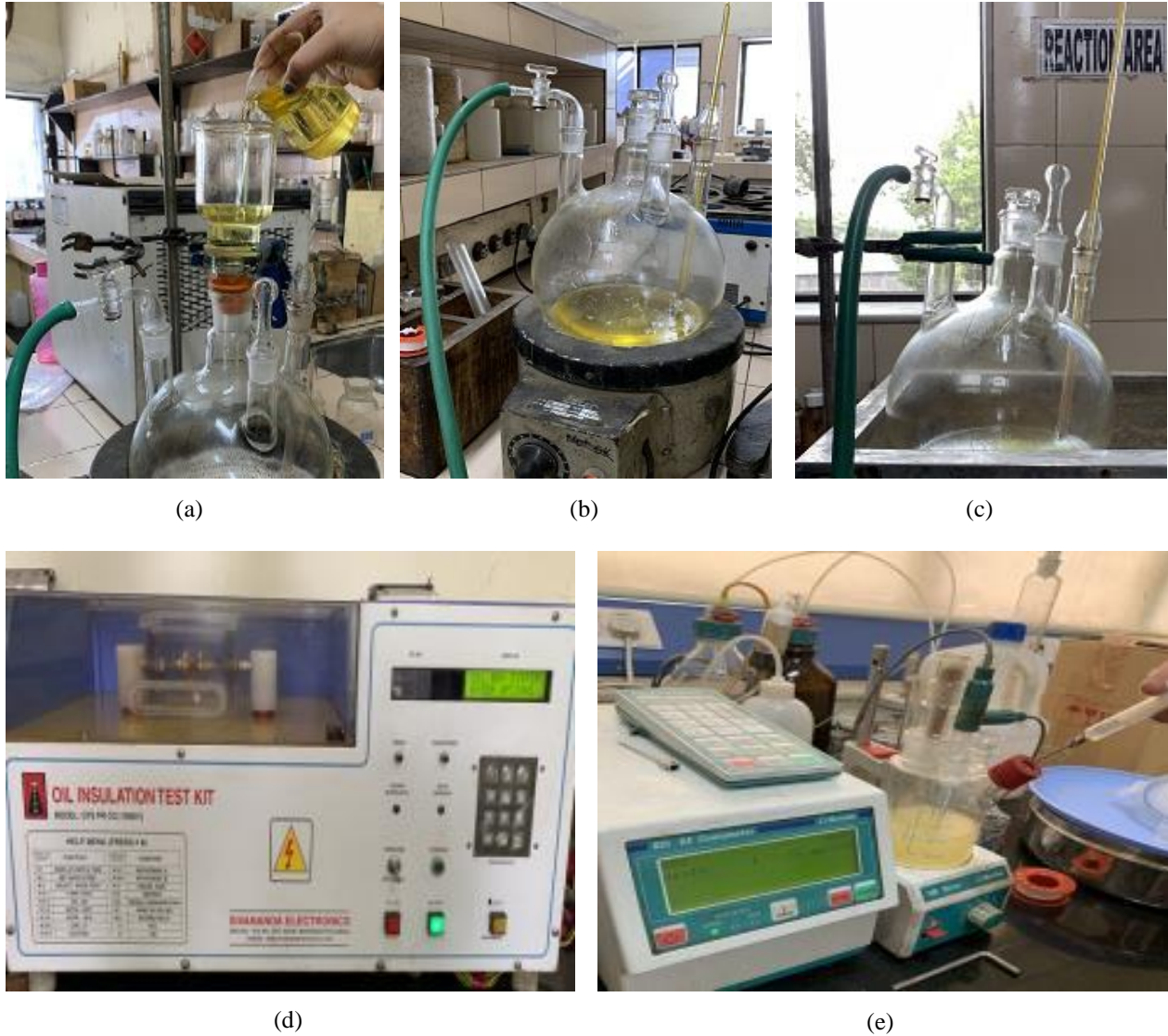
Figure 3.7: Preprocessing procedure of liquid (a) Filtering (b) Dehydration (c) Cooling (d) AC breakdown test setup (e) Moisture content measurement
