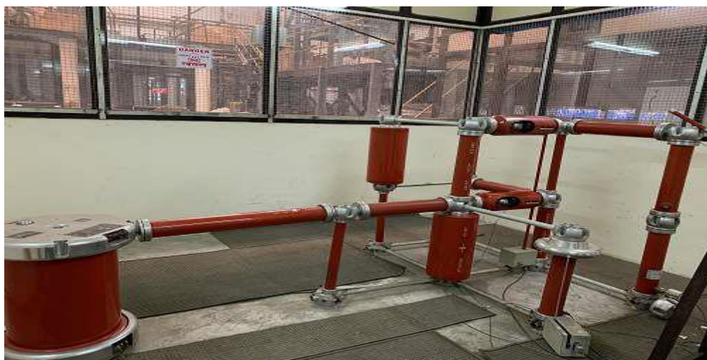
Figure 3.2: Impulse generator test setup
