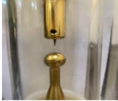
Figure 3.5: Needle-sphere electrode configuration
