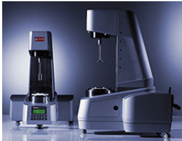
Fig 1.11: Rheometer with cylinder measuring system (left) and cone/plate measuring system (right)
