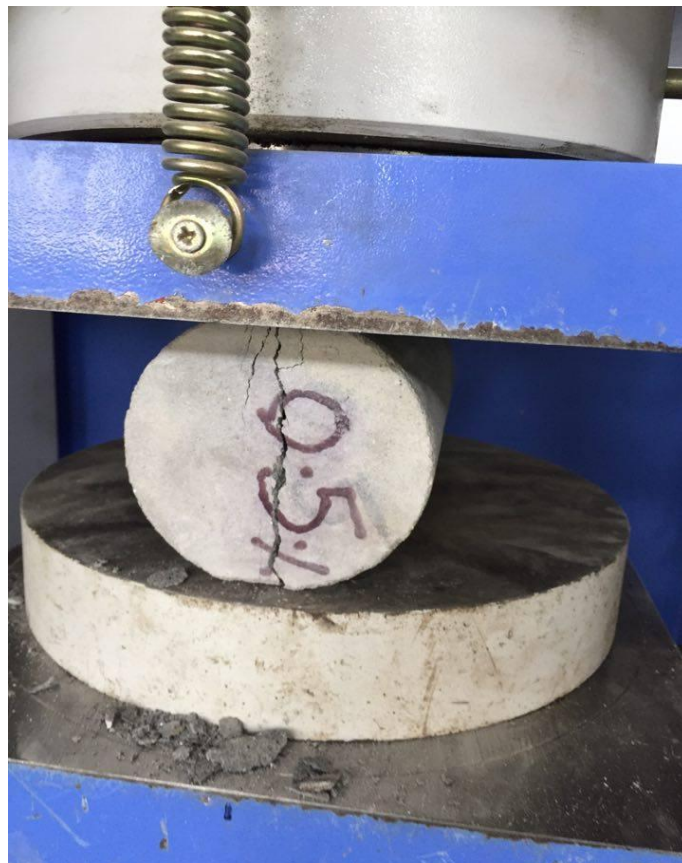
Figure 3.3 Split Tensile Test under Automated Compression Testing Machine
