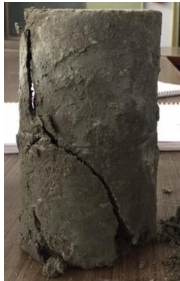
TYPE 2 FAILURE (0.5%, 1.5% and 2% Seaweed Powder)
