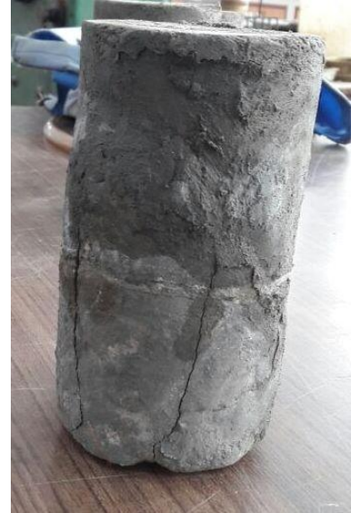
TYPE 3 FAILURE (1% Seaweed Powder)
