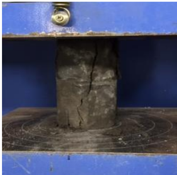
Figure 3.8 Slant Shear Test in ACTM
