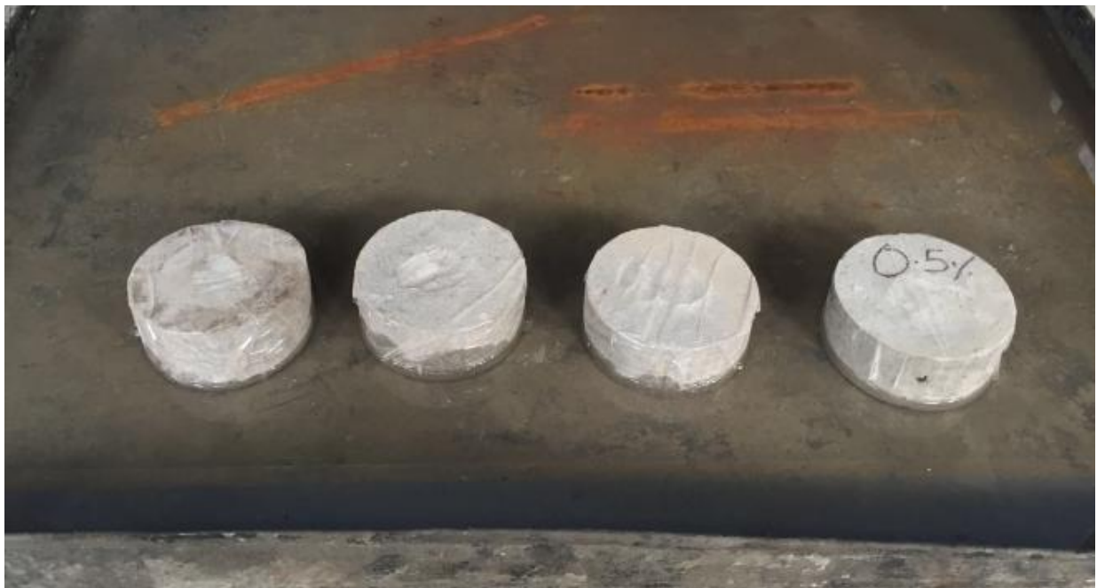
Figure 3.4. Sample Testing For Water Sorptivity.
