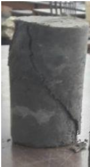
TYPE 1 FAILURE (Control Mix)
