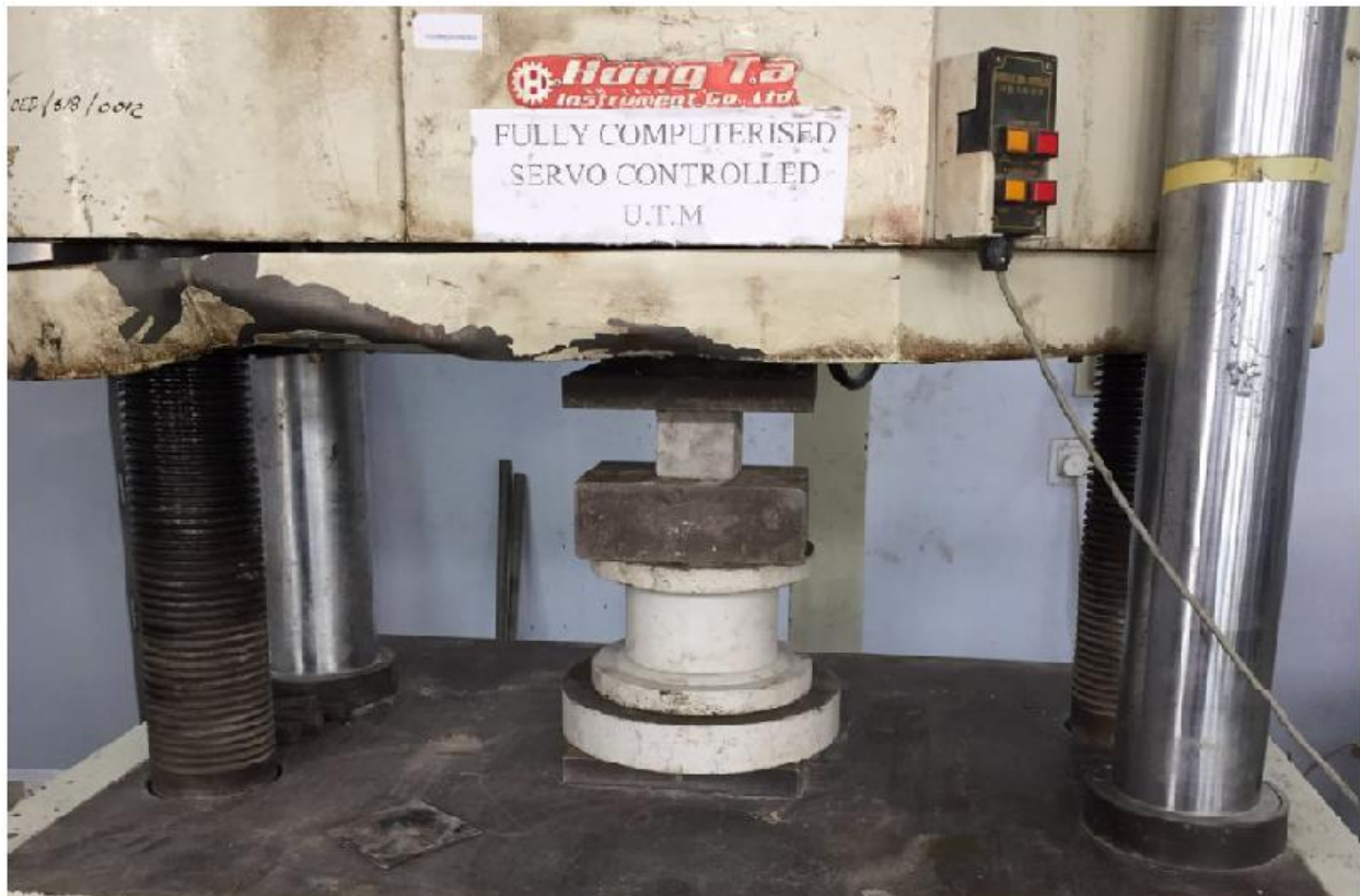
Figure 3.2 Compressive Strength of Mortar under Universal Testing Machine.
